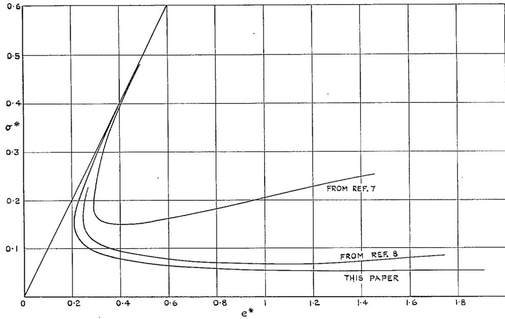
FIG. 2. Comparison of stress-strain characteristics for an ideal cylinder.
