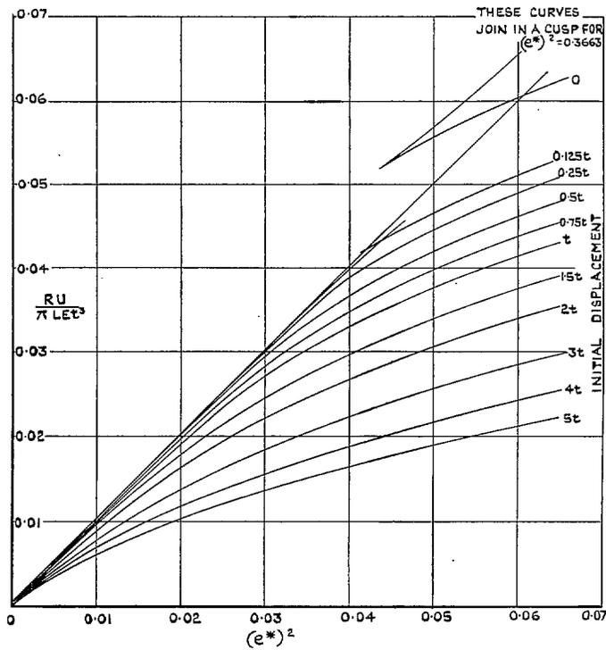
FIG. 11. Variation of strain energy with strain for varying initial displacement.
