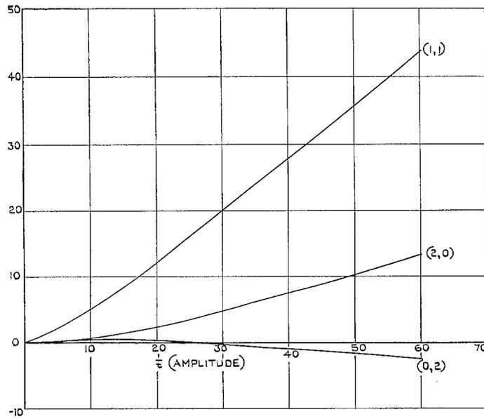
FIG. 3. Modal parameters for ideal cylinder for  $m + n = 2$ .
