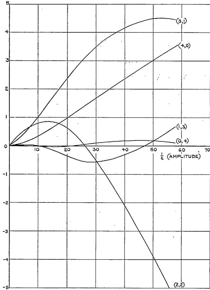
FIG. 4. Modal parameters for ideal cylinder for  $m + n = 4$ .
