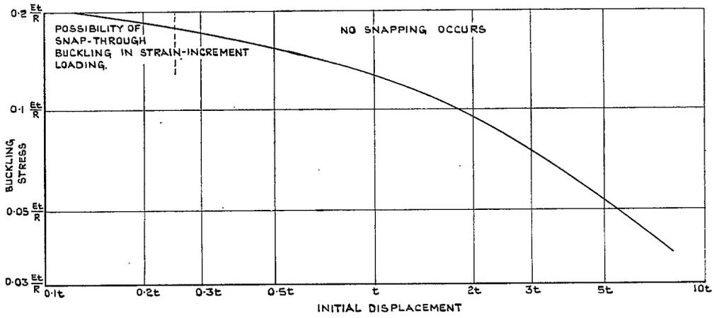
FIG. 10. Variation of buckling stress with initial displacement of imperfect cylinder.
