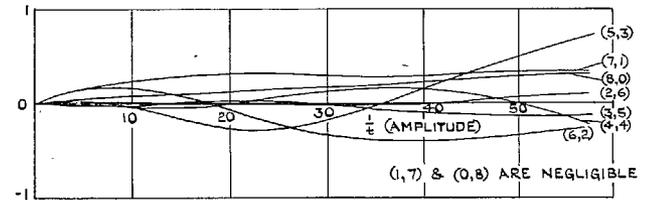
FIG. 6. Modal parameters for ideal cylinder for  $m + n = 8$ .
