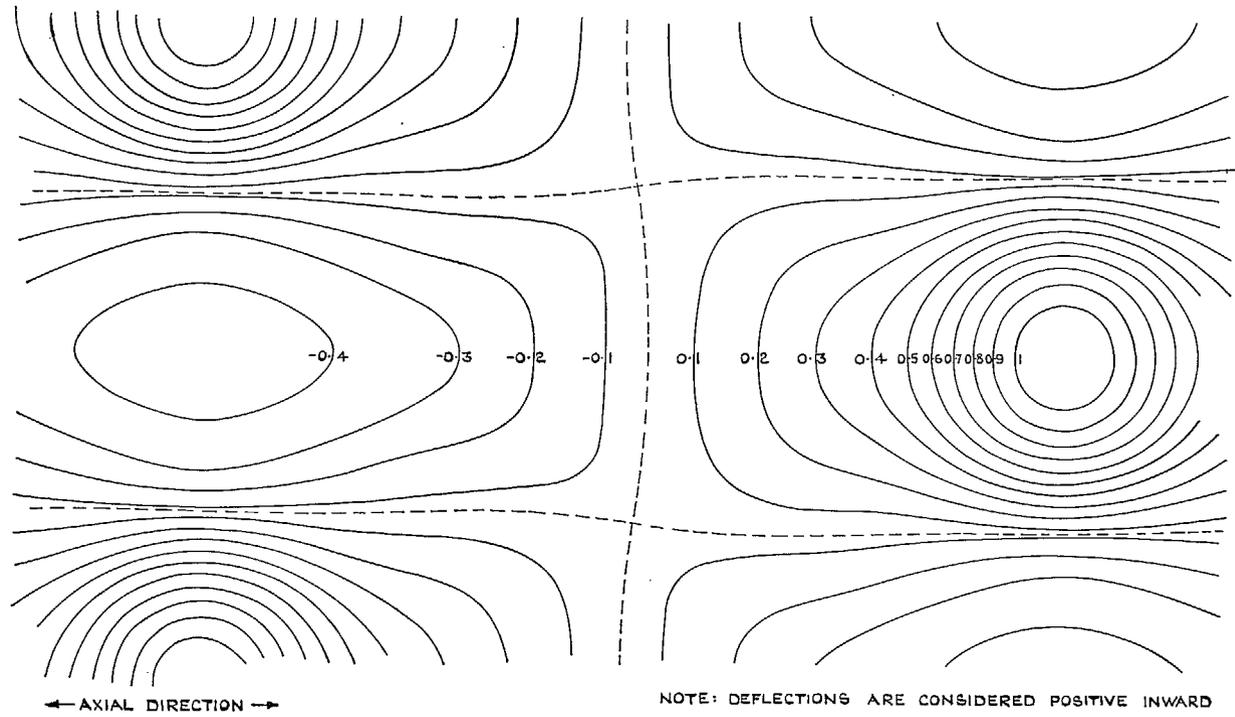
FIG. 7. Contours of deflected cylinder in region of minimum post-buckled strain.
