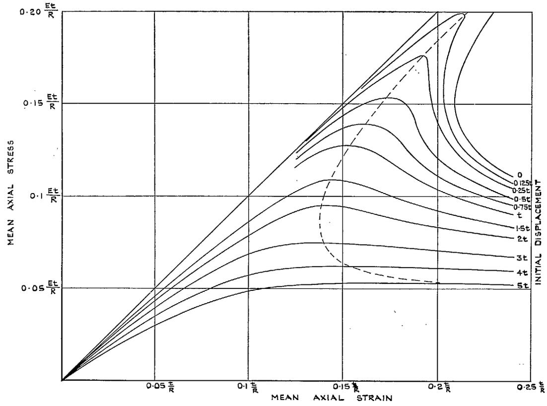
FIG. 8. Stress-strain characteristics for cylinders with initial displacement.
