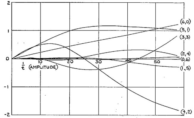
FIG. 5. Modal parameters for ideal cylinder for  $m + n = 6$ .
