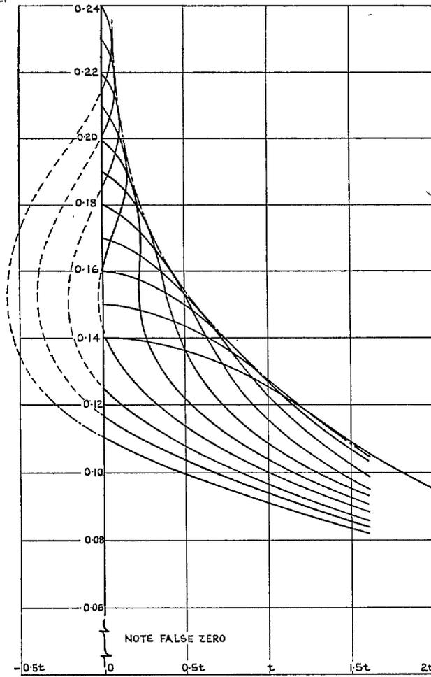
FIG. 9. Generation of buckling stress: initial displacements envelope for small initial displacements.
