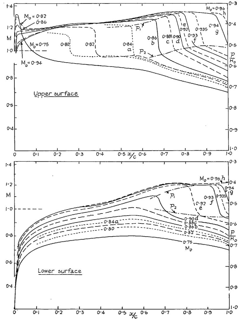
FIG. 30. Observations for a 6 per cent thick RAE 104 airfoil at 2-deg incidence; surface-pressure distributions (See also Figs. 31 to 34).
