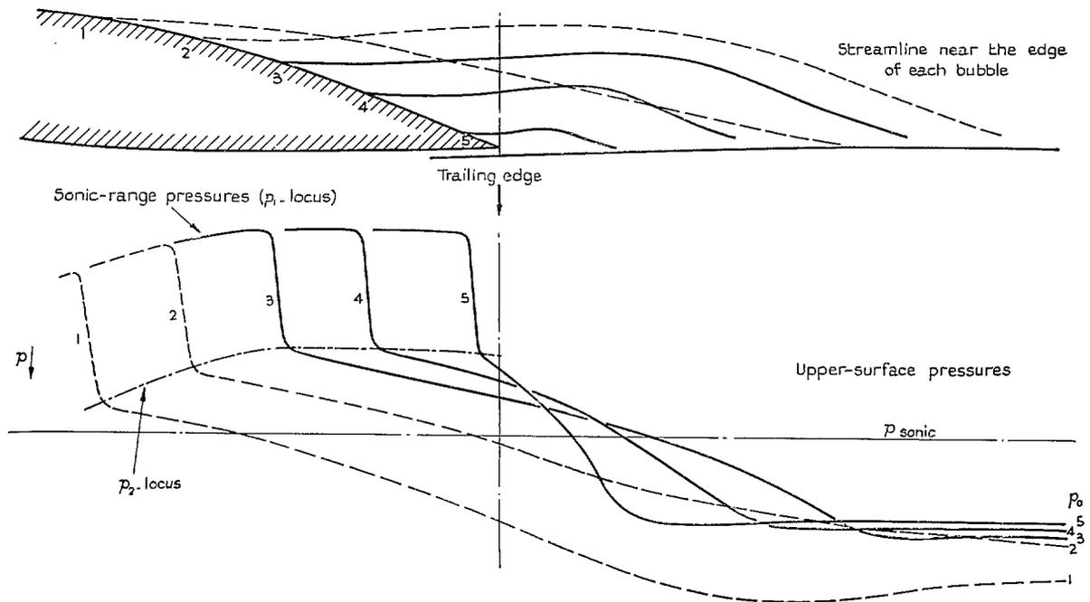
FIG. 28. Sketches to illustrate probable successive stages in the collapse of the separation 'bubble' as the upper-surface shock approaches the trailing edge.
