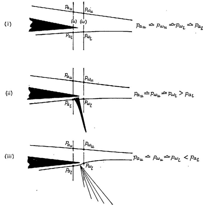
FIG. 23. Pressures at points immediately upstream and immediately downstream of the trailing edge.
