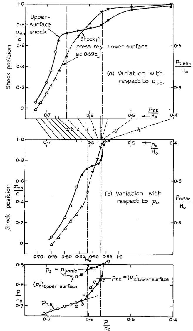
FIG. 33. Observations for a 6 per cent thick RAE 104 aerofoil at 2-deg incidence; variation of a flow parameter (shock position or pressure at a fixed point) for each surface (See also Figs. 30, 31, 32 and 34).
