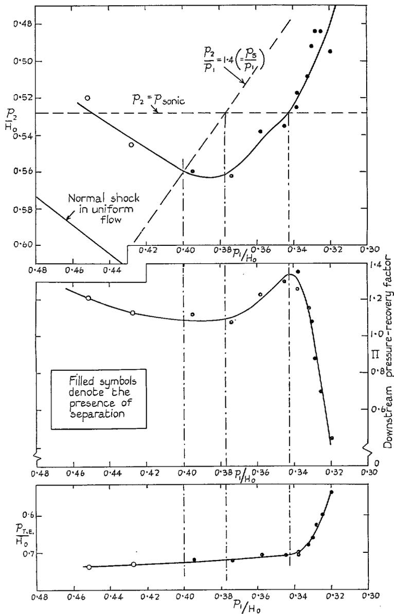
FIG. 7. Variation with shock upstream pressure  $p_1$  of certain quantities derived from the upper-surface pressure distribution (for definitions see Fig. 6) (10 per cent thick RAE 102 aerofoil at 2-deg incidence).
