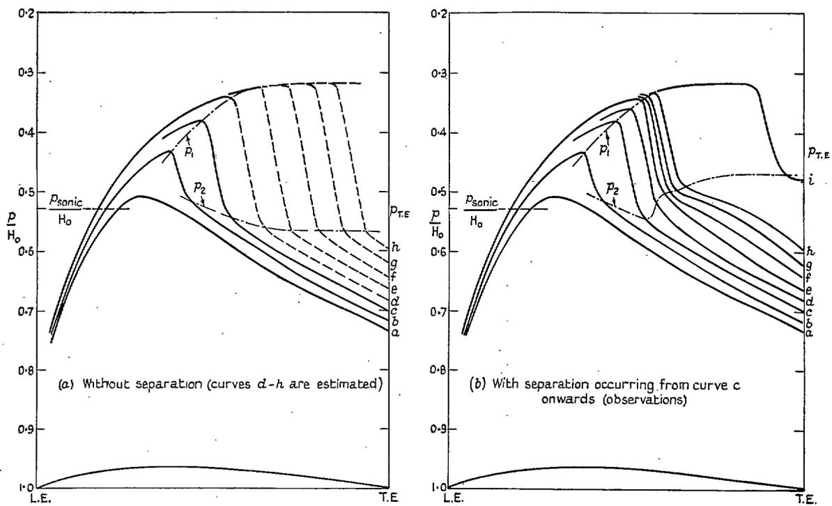
FIG. 12. Surface-pressure distributions showing the movement of the shock for a prescribed variation in trailing-edge pressure (See Fig. 13 for shock position plotted against  $p_{T,E}/H_0$ ).
