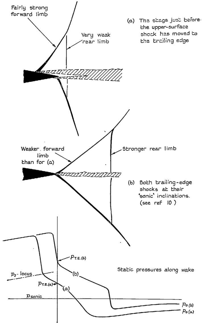
FIG. 29. Movement of the shocks into their 'sonic' positions and inclinations.
