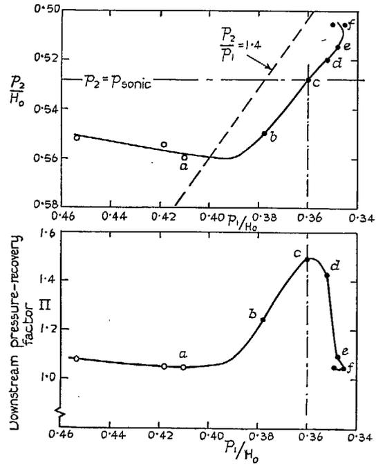
FIG. 32. Observations for a 6 per cent thick RAE 104 aerofoil at 2-deg incidence; quantities derived from the upper-surface pressures (See also Figs. 30, 31, 33 and 34). (Filled symbols denote the presence of separation.)
