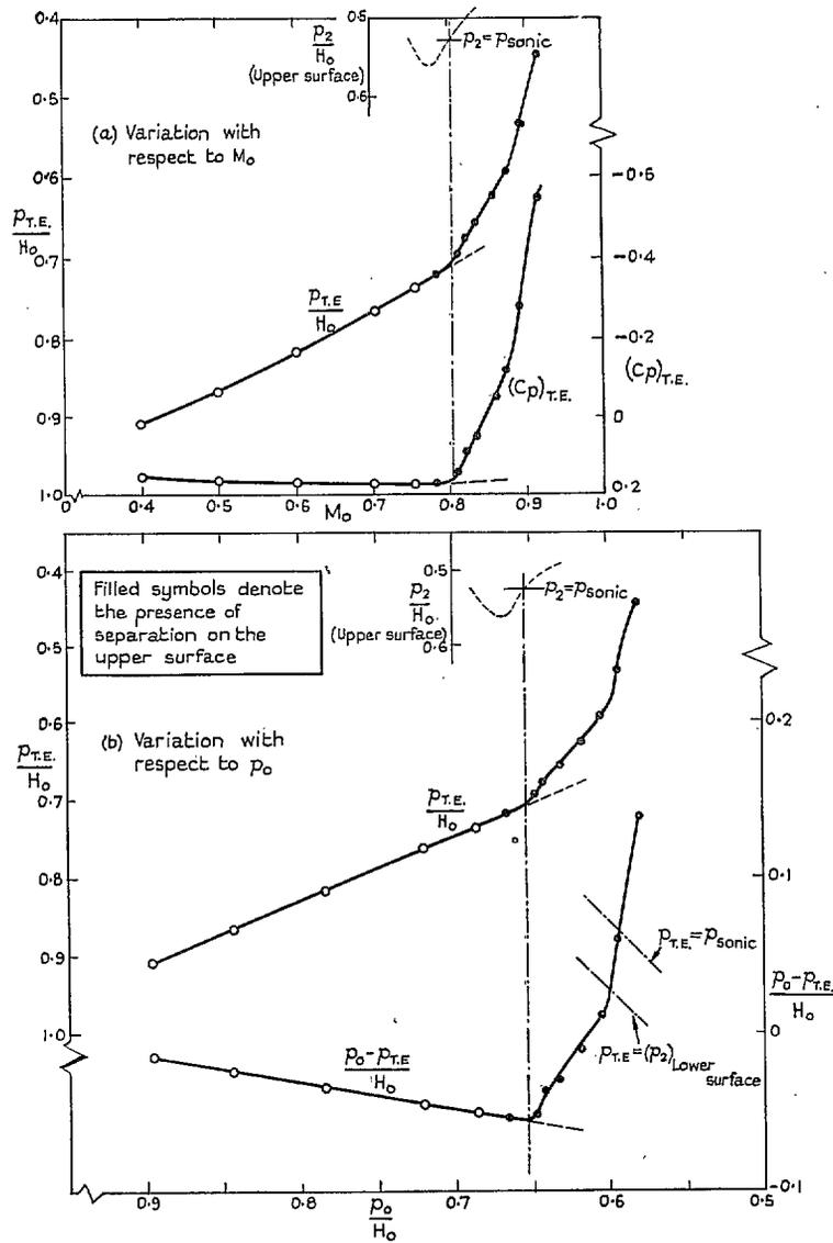
FIG. 15. Variation of trailing-edge pressure  $p_{T.E.}$  for fixed incidence; different methods of plotting to show the divergence from the normal (pre-separation) variation (10 per cent thick RAE section at 2-deg incidence).
