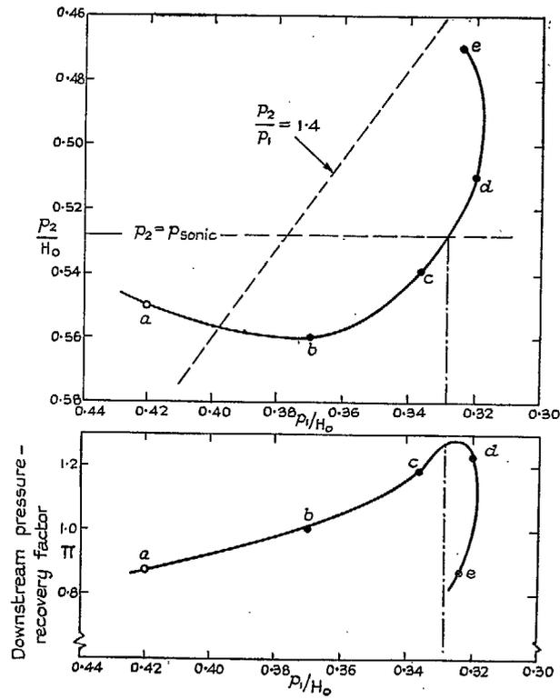
FIG. 42. Observations for a 6 per cent thick RAE 104 aerofoil through a range of incidence;  $M_0 = 0.75$ ; quantities derived from the upper-surface pressures (See also Figs. 40, 41 and 43) (Filled symbols denote the presence of separation).
