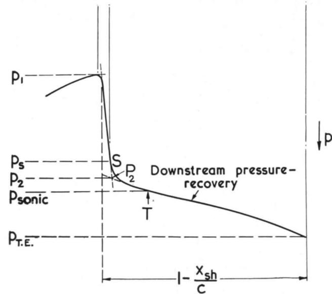
FIG. 6. Details of the flow and surface-pressure distribution near and downstream of separation; definition of certain pressures.
