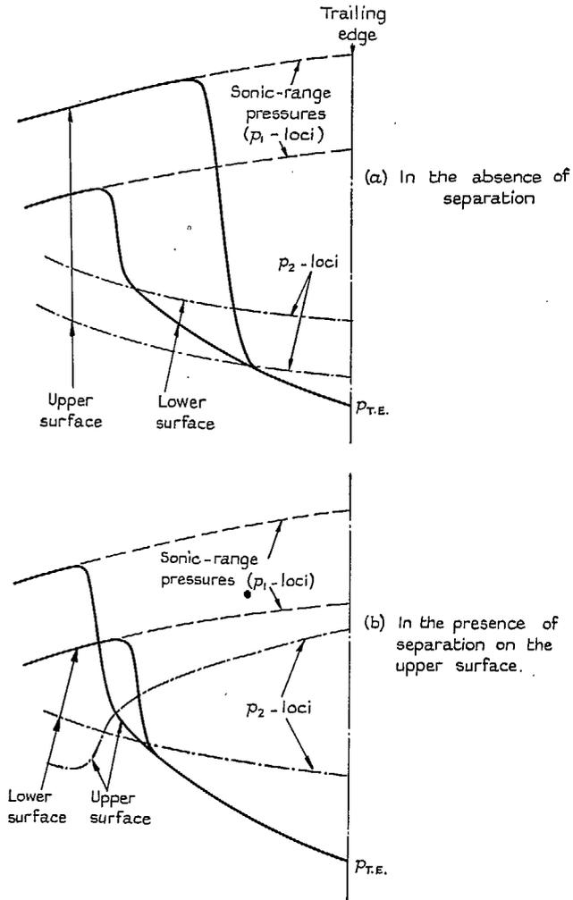
FIG. 22. Sketches of surface-pressure distributions to show relative shock positions for an aerofoil at a fairly low incidence and a Mach number close to unity.
