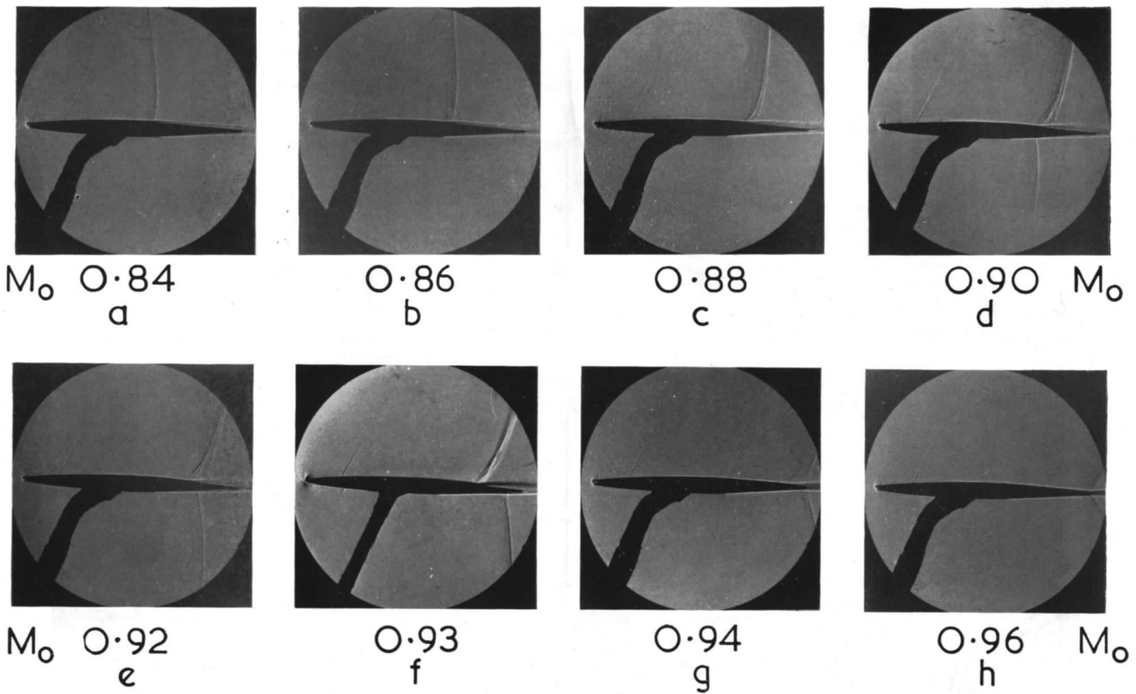
FIG. 31. Observations for a 6 per cent thick RAE 104 aerofoil at 2-deg incidence; flow photographs (See also Figs. 30 and 32 to 34).
