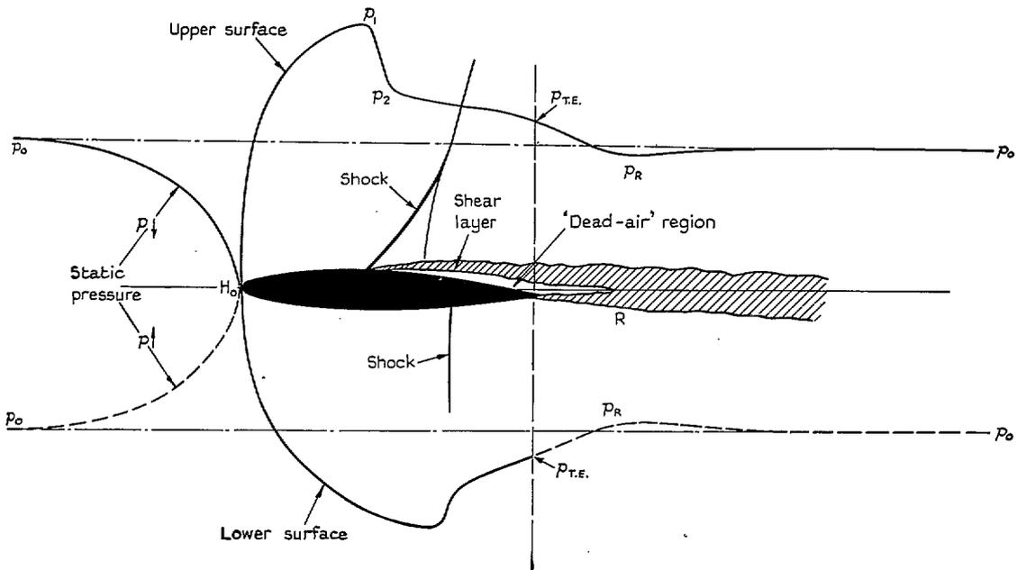
FIG. 3. Sketch of certain features of the flow about an aerofoil and along its wake in the presence of shock-induced separation on the upper surface.
