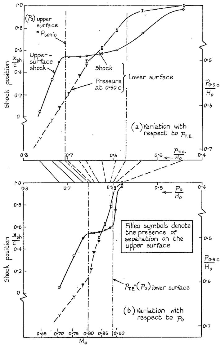
FIG. 17. Variation of a flow parameter for each surface of an aerofoil to show the rate of development of the flow on the two surfaces relative to one another (both diagrams) and with respect to the free-stream static pressure (lower diagram only) (10 per cent thick RAE 102 section at 2-deg incidence).
