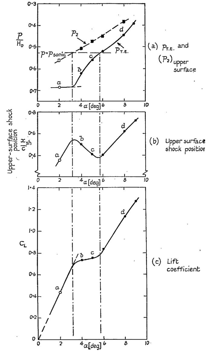
FIG. 46. Observations for a 6 per cent thick aerofoil through a range of incidence at  $M = 0.8$  (See also Fig. 45) (Filled symbols denote the presence of separation).
