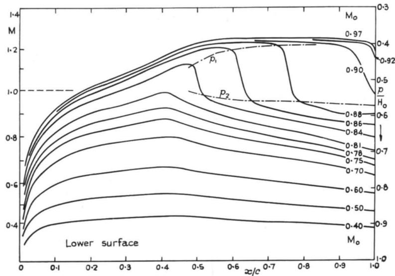
FIG. 1. Surface pressure distributions for a symmetrical aerofoil at a fixed positive incidence (10 per cent thick RAE 102 section at 2-deg incidence).
