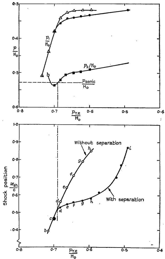
FIG. 13. Variation of shock position with trailing-edge pressure (See Fig. 12 for corresponding pressure distributions).
