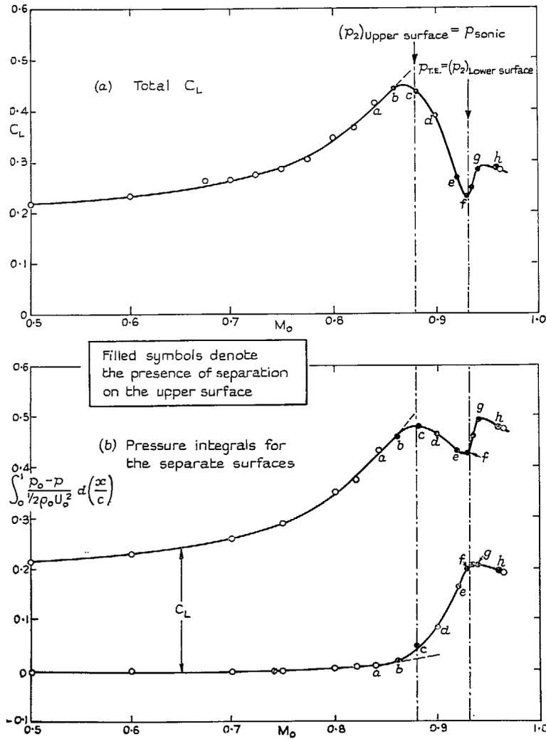
FIG. 34. Observations for a 6 per cent thick RAE 104 aerofoil at 2-deg incidence; variation with free-stream Mach number of the total  $C_L$  and of the contributions from the separate surfaces (See also Figs. 30 to 33).
