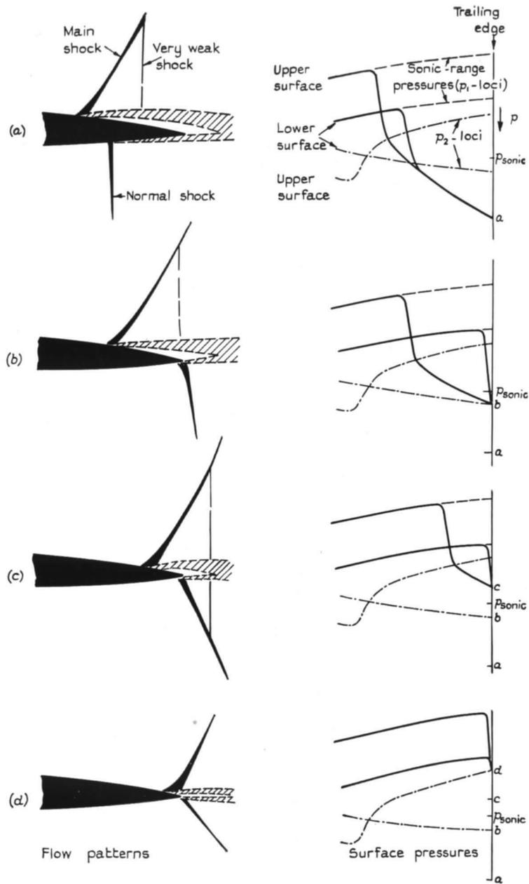
FIG. 24. Sketches to illustrate the changes in the flow on the two surfaces of an airfoil relative to one another once the lower-surface shock has reached the trailing edge.
