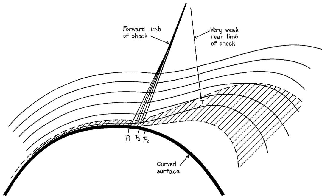
FIG. 8. Diagrammatic sketch of streamlines and boundary flow near separation on a curved surface (curvature greatly exaggerated).  $T$  is the approximate position at which the velocity along the streamline has fallen to the sonic value.
