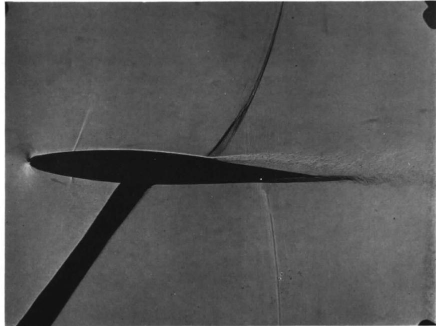
FIG. 2. Schlieren photograph of the flow past an aerofoil with severe separation at the foot of the upper-surface shock; 10 per cent RAE 102 section at 2-deg incidence ( $M_0 = 0.88$ ).
