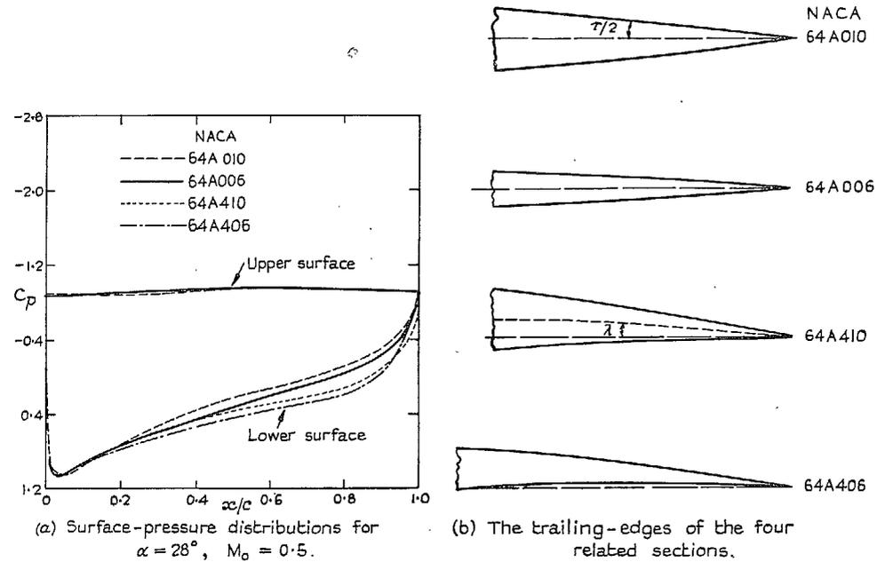
FIG. 21. The influence of trailing-edge angle and camber on the pressures over the lower surface in the presence of severe separation on the upper surface (results for four related NACA sections; Ref. 23).
