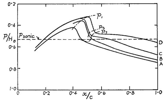
FIG. 10. Surface-pressure distributions, and quantities derived therefrom, at stages in the development of the separated flow (8 per cent thick half-aerofoil) (See Fig. 11 for corresponding flow photographs).
