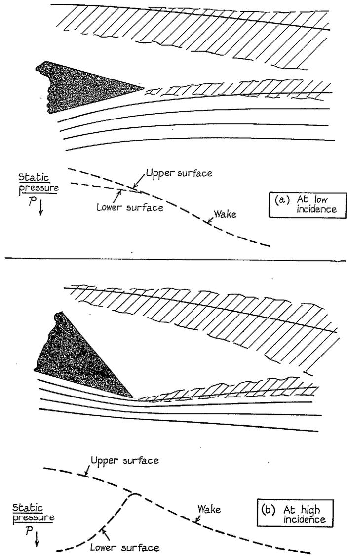
FIG. 20. Sketches to illustrate the influence of the upper-surface separation on the flow near the trailing edge on the lower surface; low and high incidence.
