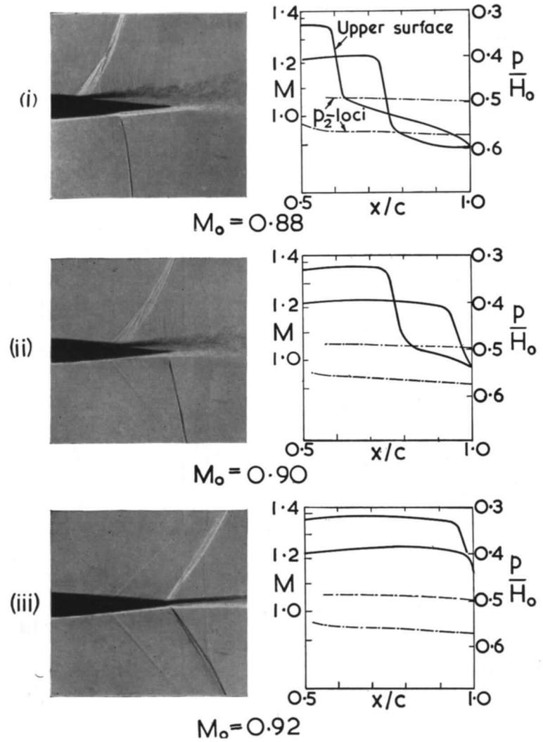
FIG. 25. Observations showing the changes in the flow on the two surfaces of an airfoil relative to one another once the lower-surface shock has reached the trailing edge (10 per cent RAE 102 section at 2-deg incidence) (See sketches in Fig. 24).
