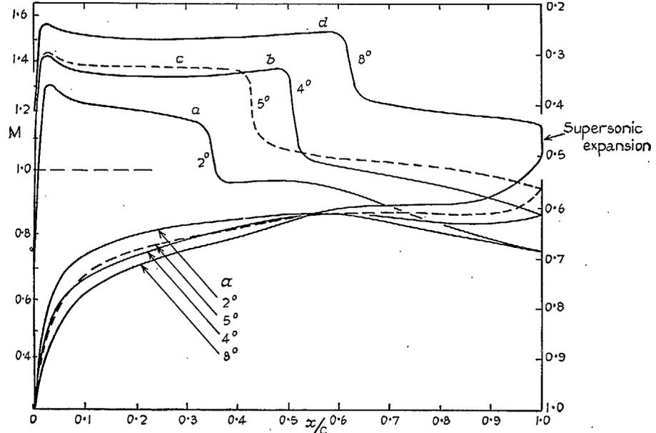
FIG. 45. Observations for a 6 per cent thick aerofoil through a range of incidence at  $M_0 = 0.8$  (See also Fig. 46).
