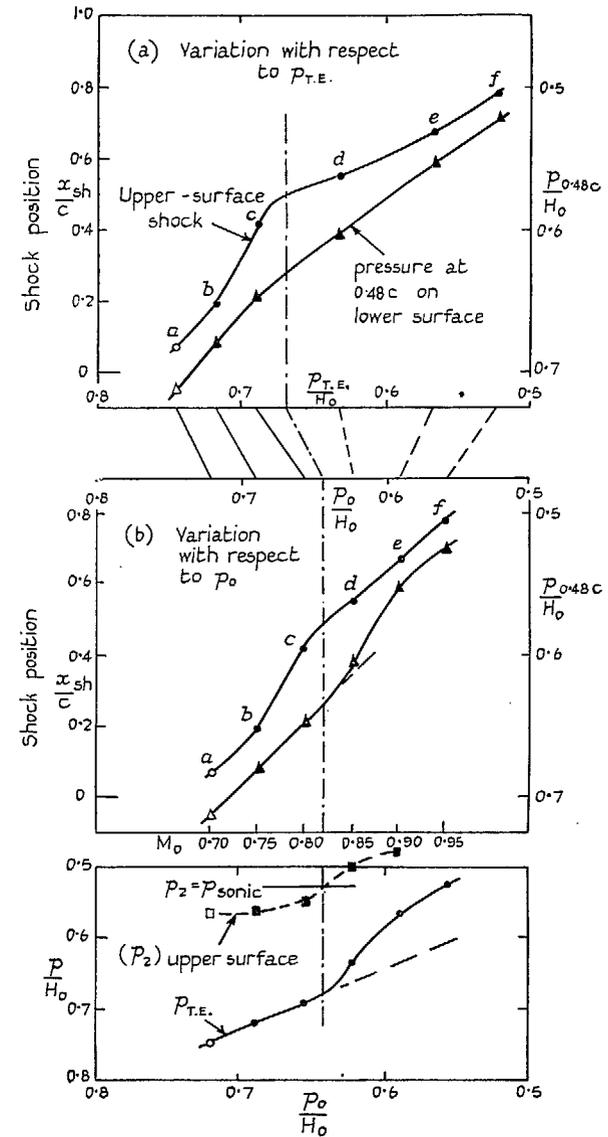
FIG. 38. Observations for a 6 per cent thick RAE 104 aerofoil at 3.7-deg incidence; variation of a flow parameter (shock position and pressure at a fixed point) for each surface (See also Figs. 35, 36, 37 and 40).
