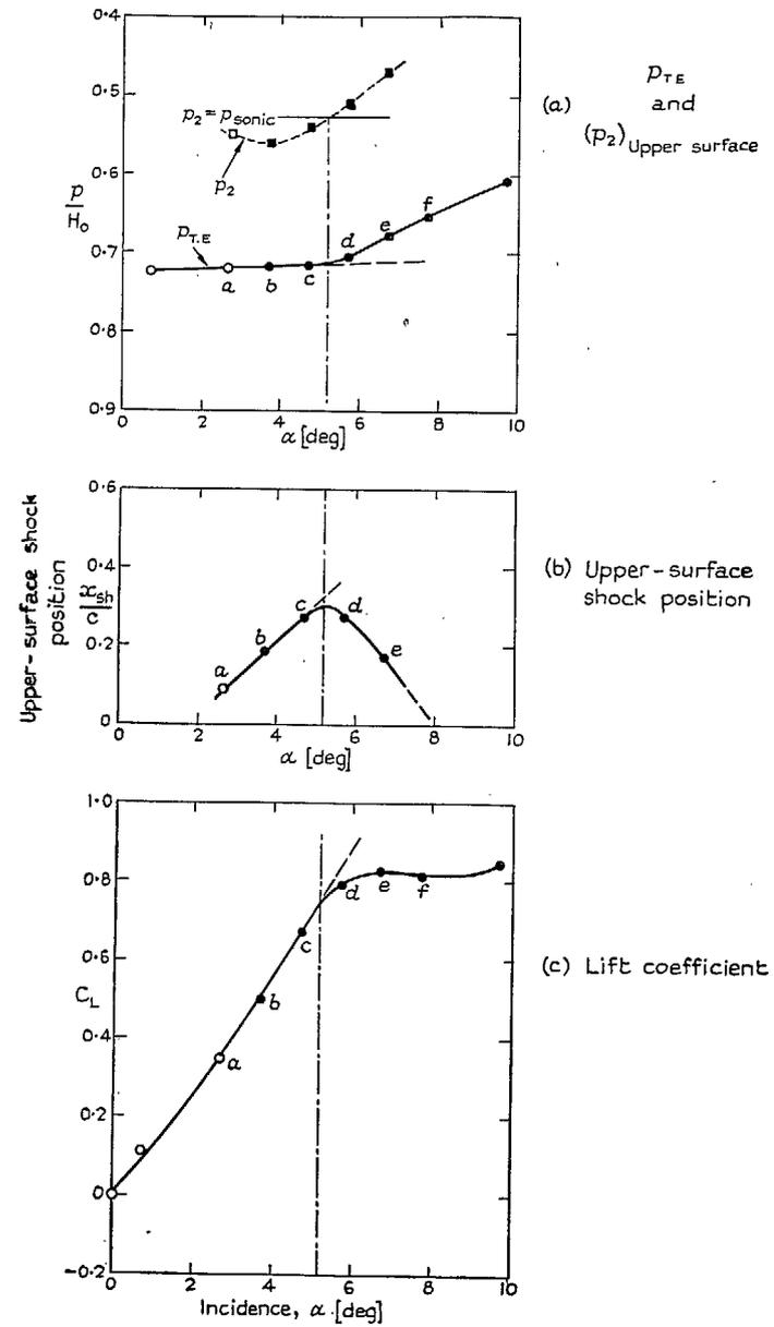
FIG. 43. Observations for a 6 per cent thick RAE 104 aerofoil through a range of incidence;  $M_0 = 0.75$  (See also Figs. 40, 41 and 42) (Filled symbols denote the presence of separation).
