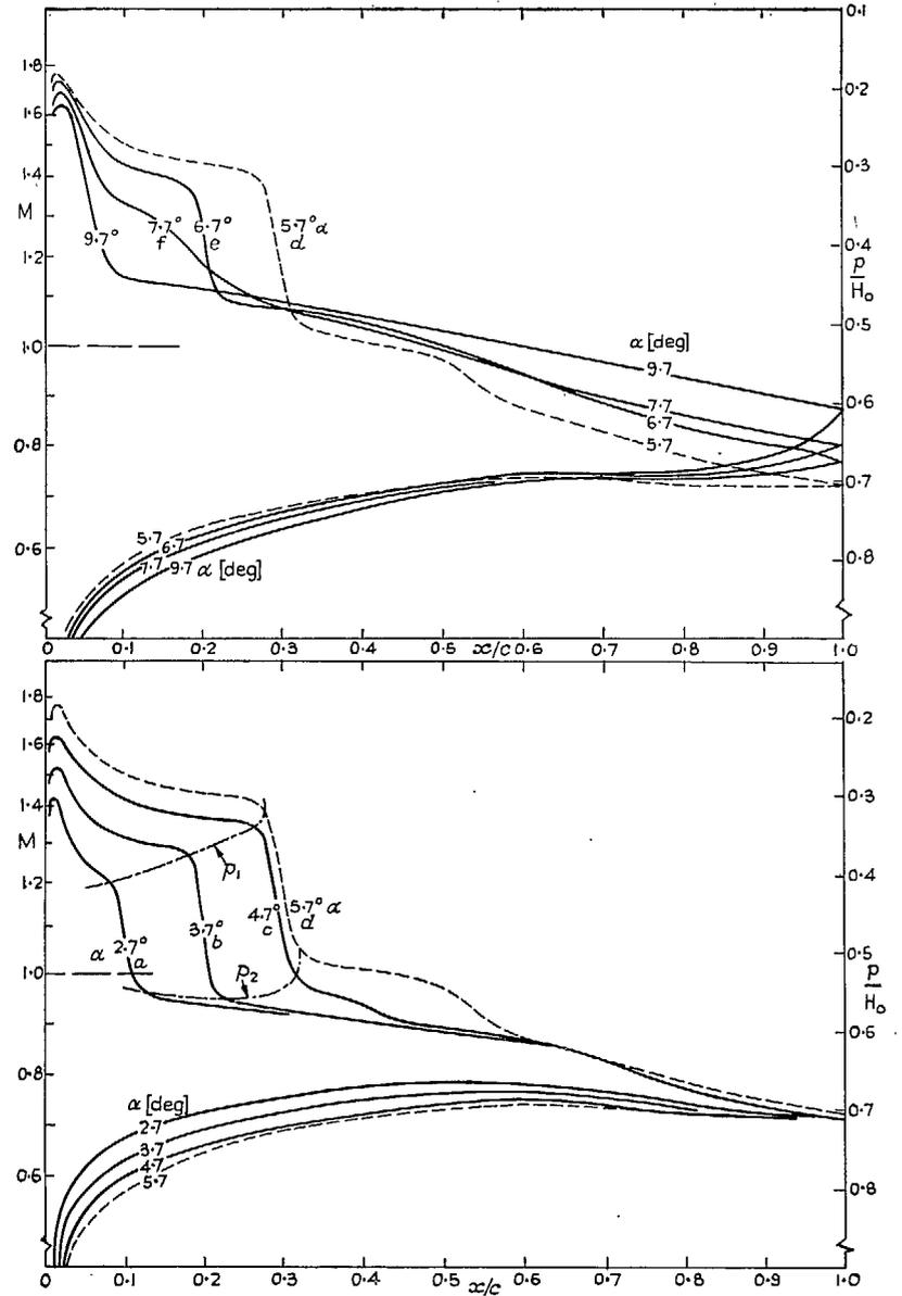
FIG. 40. Observations for a 6 per cent thick RAE 104 aerofoil through a range of incidence;  $M_0 = 0.75$ ; surface-pressure distributions (See also Figs. 41 to 43).
