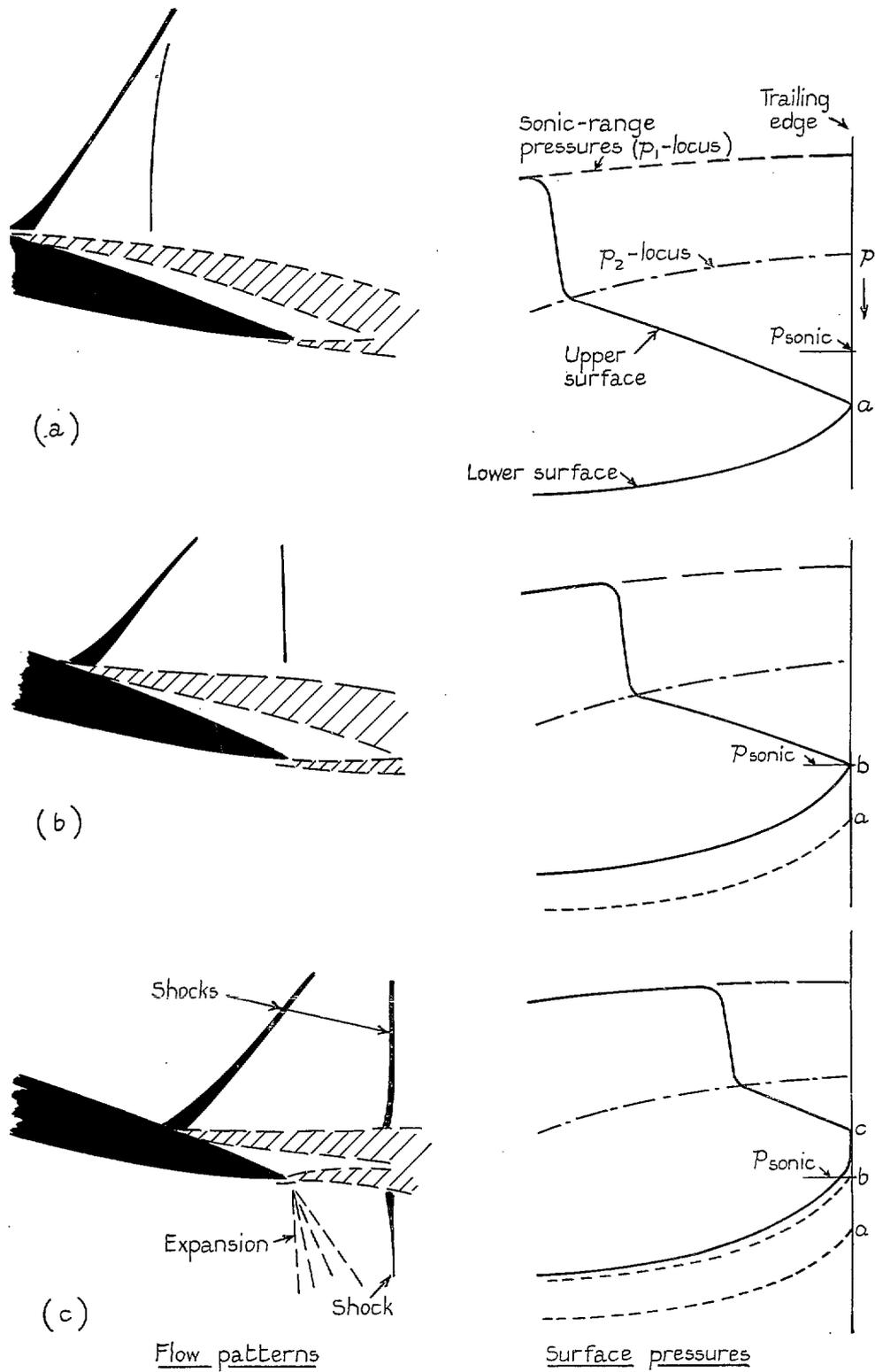
FIG. 26. Sketches to illustrate the changes in the flow on the two surfaces of an airfoil relative to one another once a supersonic expansion can occur at the trailing edge on the lower surface.
