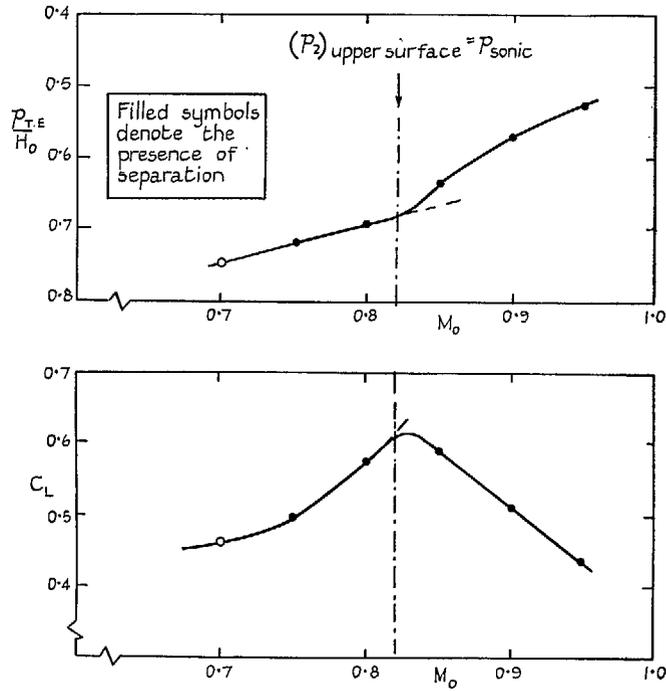
FIG. 39. Observations for a 6 per cent thick RAE 104 aerofoil at 3.7-deg incidence; variation with free-stream Mach number of  $C_L$  and  $p_{T,E}$  (See also Figs. 35 to 38).
