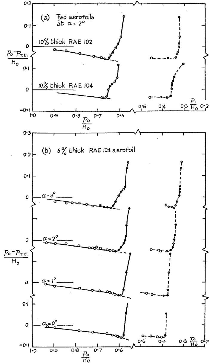
FIG. 18. Effect of section shape and aerofoil incidence on the variation of trailing-edge pressure (Filled symbols denote the presence of separation on the upper surface).
