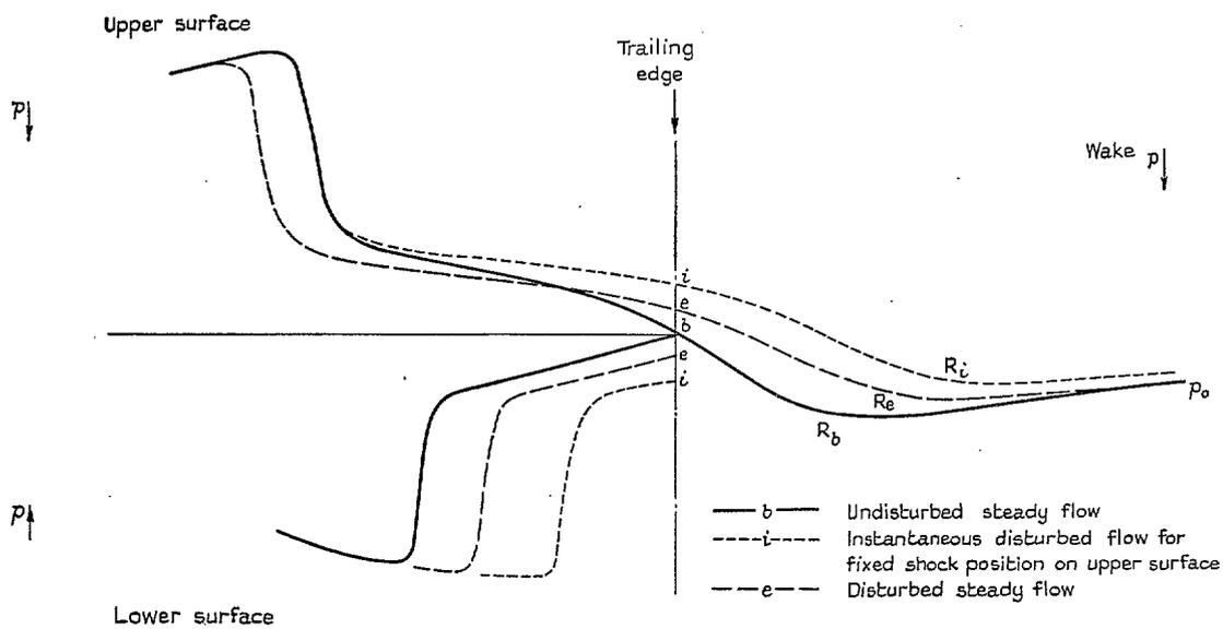
FIG. 16. Sketch of pressure distributions over the rear of an airfoil and along the wake to illustrate the effect of a hypothetical disturbance to the separated flow near the foot of the shock on the upper surface.
