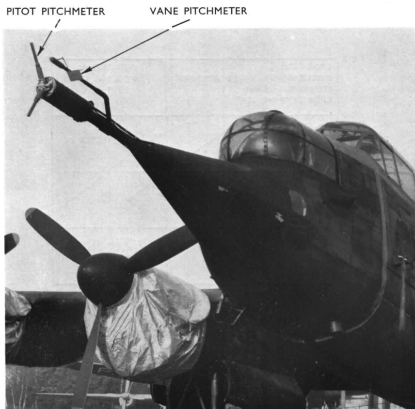
FIG. 2. Nose of Lancaster ME.540 showing the two pitchmeters.
