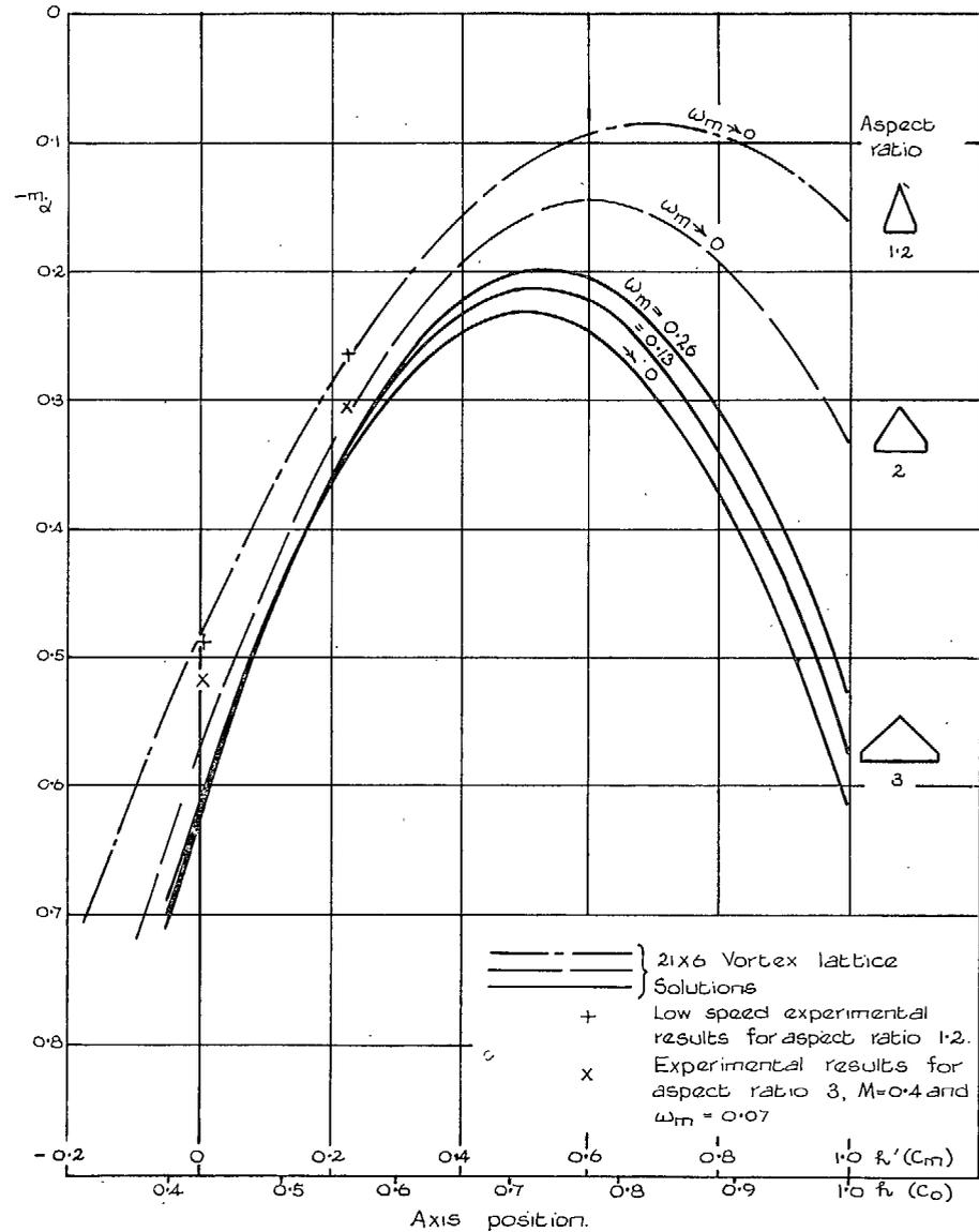
FIG. 2. Variation of  $-\dot{m}_\alpha$  with axis position—family of delta wings with taper ratio  $1/7$ .
