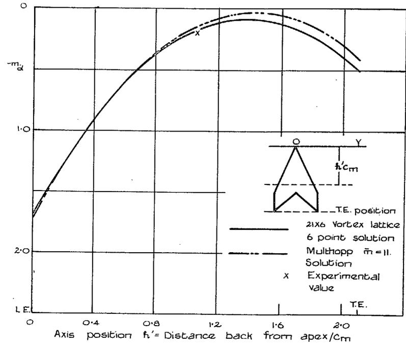
FIG. 4. Values of  $-m_\alpha$  for arrowhead wing of aspect ratio 1.32, as  $\omega_m \rightarrow 0$ .
