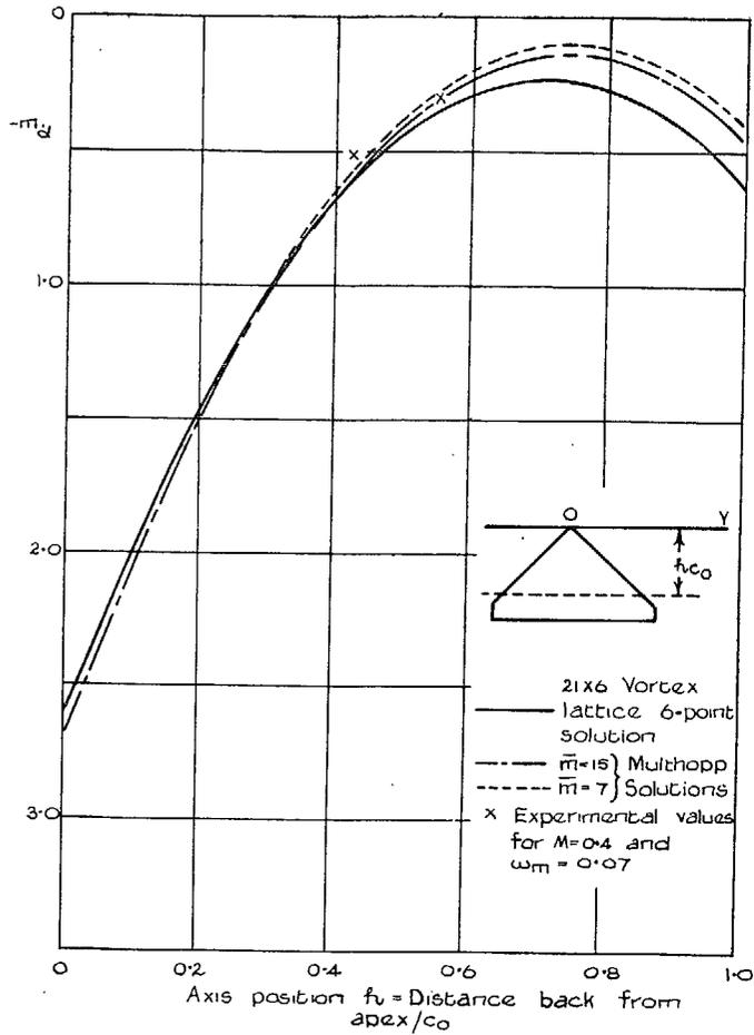
FIG. 3. Values of  $-m_\alpha$  for delta wing of aspect ratio 3 as  $\omega_m \rightarrow 0$ .
