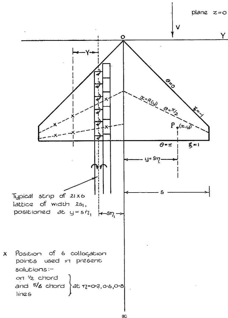
FIG. 1. Layout for  $21/6$  vortex lattice.
