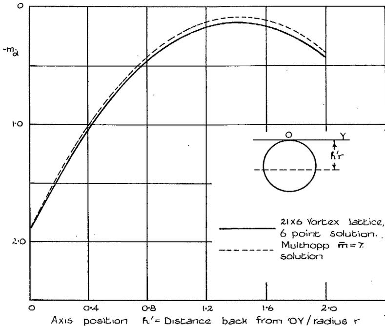
FIG. 5. Values of  $-m_{\alpha}$  for circular plate as  $\omega_r \rightarrow 0$ .
