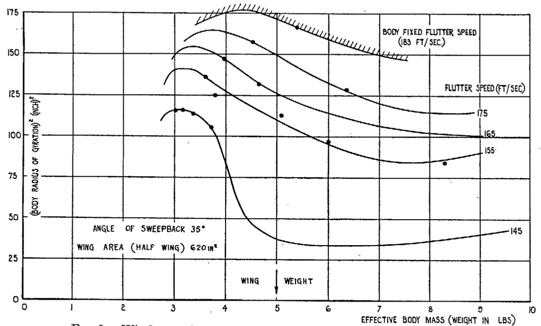
FIG. 9. Wind-tunnel results after including equivalent spring masses.
