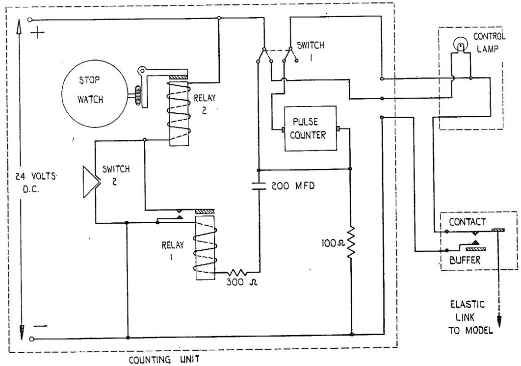
FIG. 7. Arrangement for measuring frequency.
