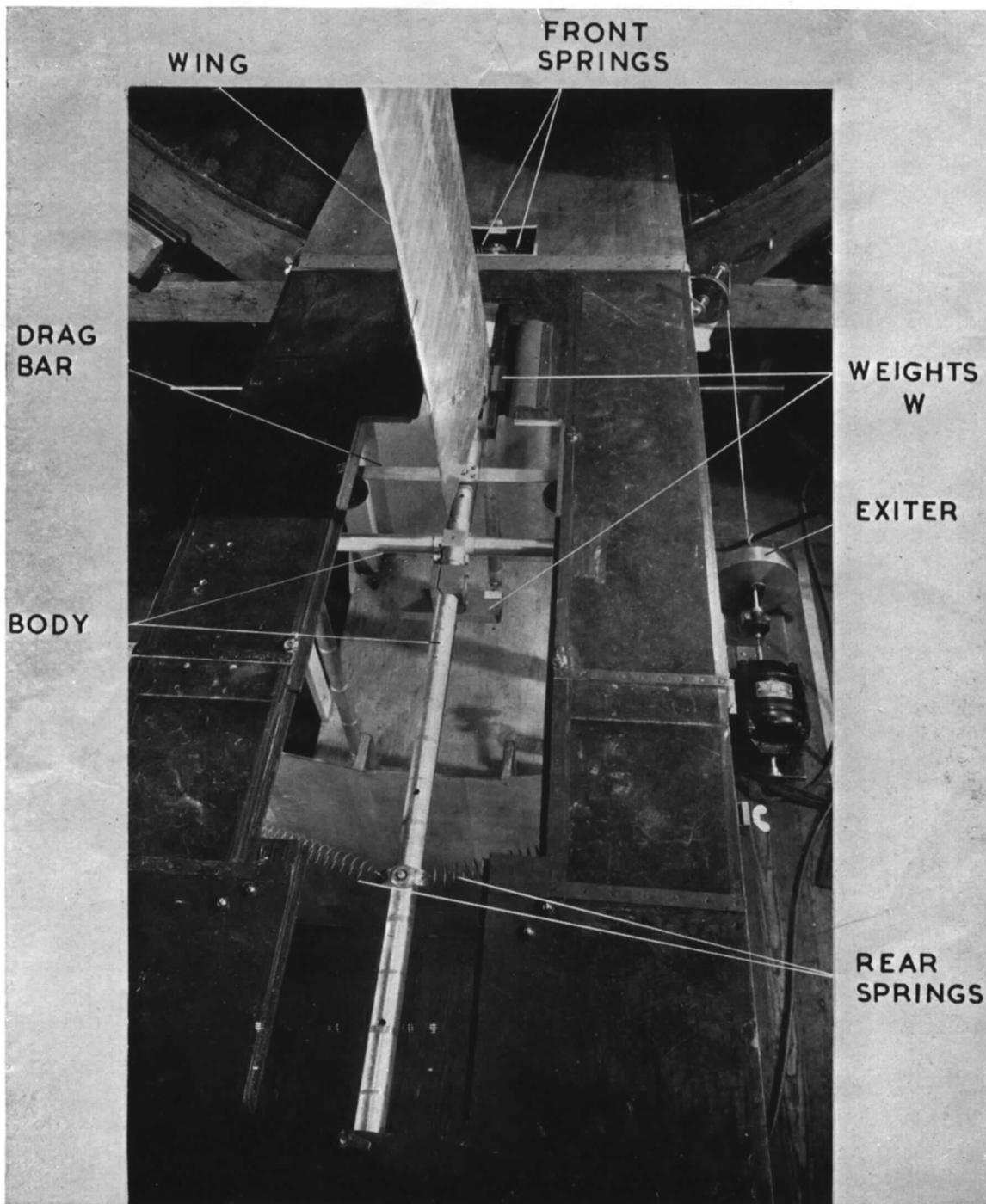
FIG. 2. Top view of flutter rig.
