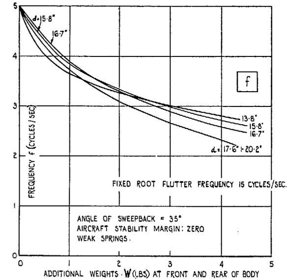
FIG. 8. Typical wind-tunnel results.
