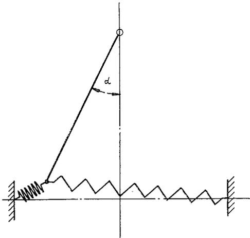
FIG. 6. Geometry of spring arrangement in pitch.
