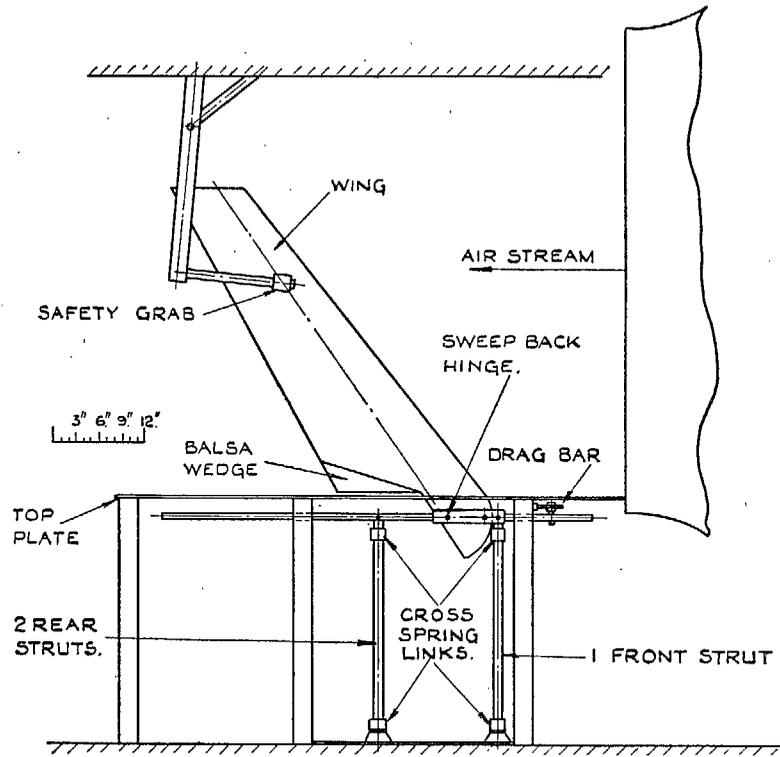
FIG. 3. General arrangement of the rig.
