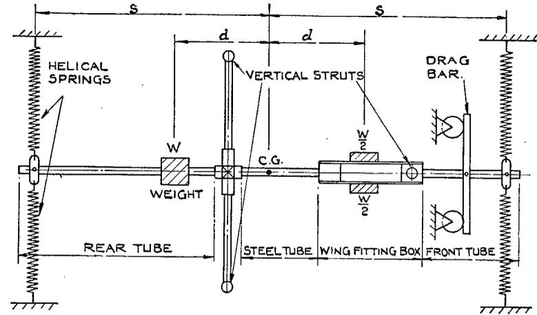
FIG. 4. Plan of body and supports—diagrammatic.
