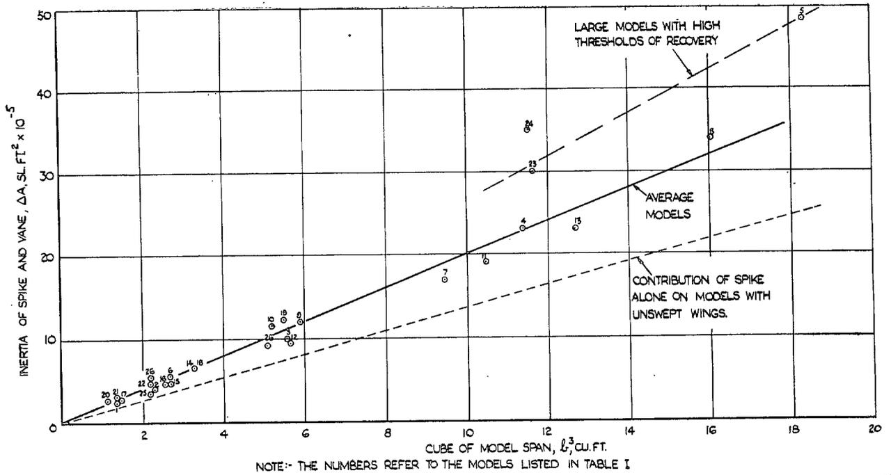
FIG. 3. Addition to rolling moment of inertia of spinning models due to a spike and vane mounted on one wing tip.
