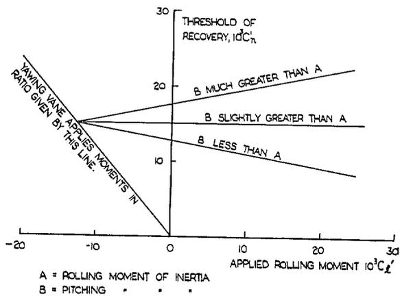
FIG. 2. Sketch showing effect of applied rolling moment on threshold of recovery.
