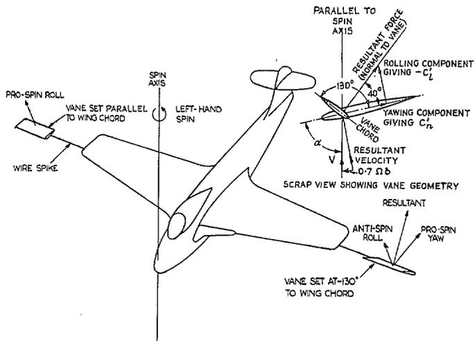
FIG. 1. Method of applying moments to spinning model.
