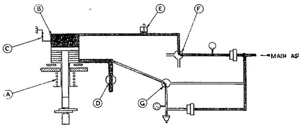
AIR IS FED TO THE BOTTOM OF THE PISTON THUS RAISING THE ELECTRODE FROM THE COMPLETED WELD
