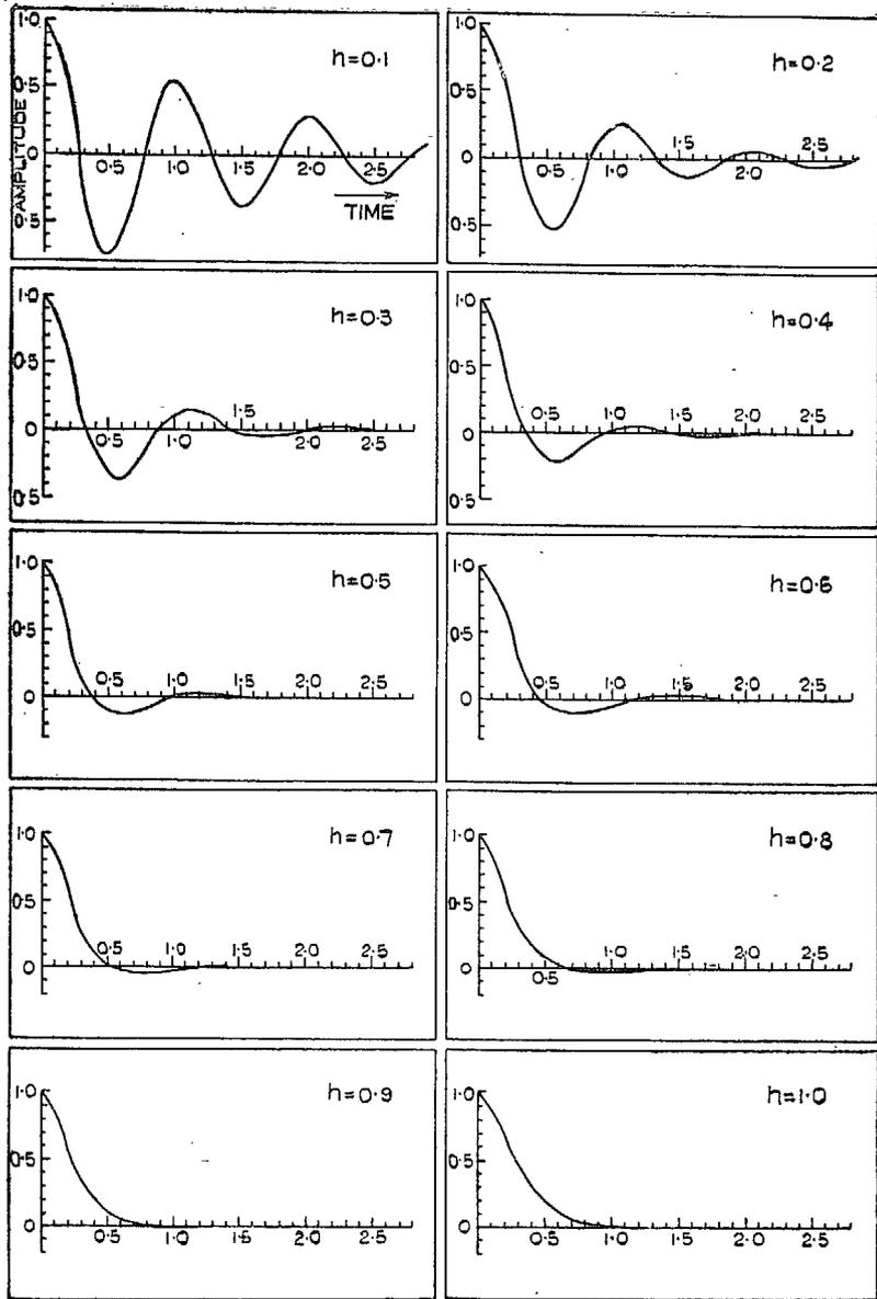
FIG. 5. Decay curves for different damping factors.
