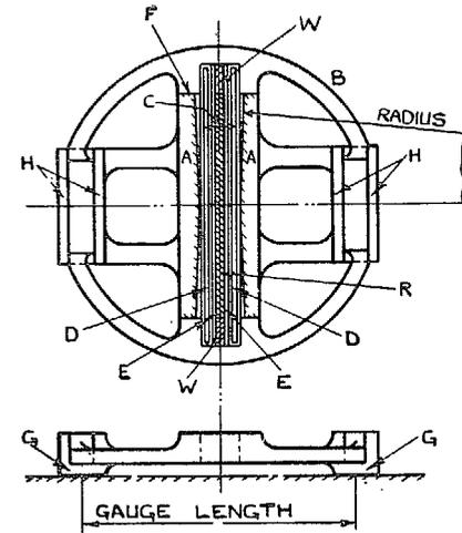
Multiple plate capacity type strain gauge.
