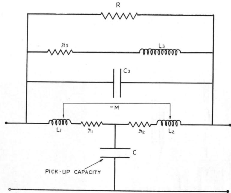
FIG. 27. Bridged-T circuit for variable capacity pick-up unit (Roess).
