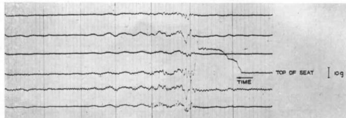
FIG. 68c. Acceleration on seat during ejection in flight.
