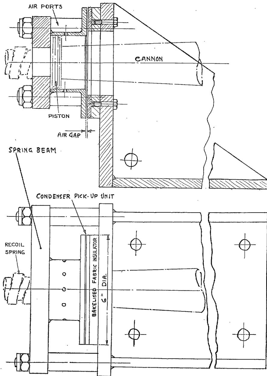
FIG. 56. Front mounting for 20 mm Hispano gun.
