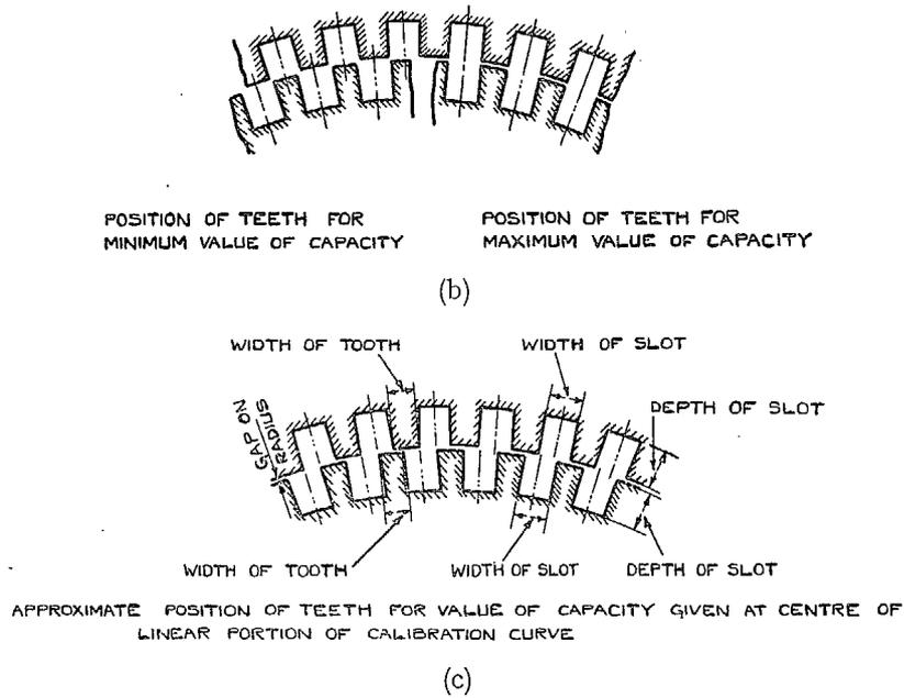
FIG. 18b and c. Enlarged view of serrations of R.A.E. capacity torsigraph.
