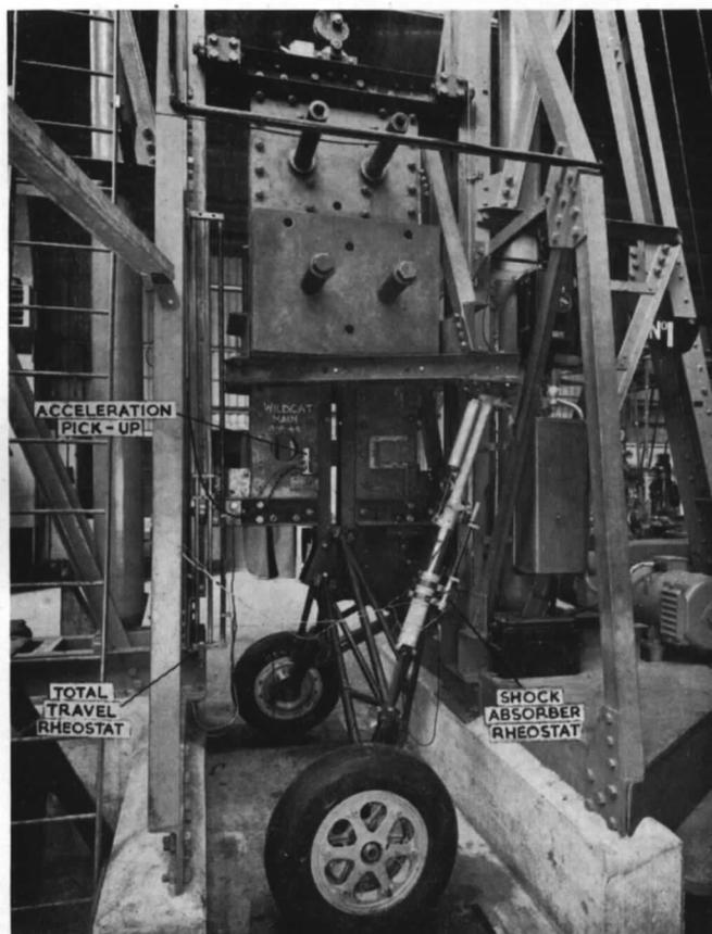
FIG. 47. Undercarriage drop testing installation.
