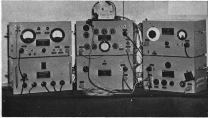
FIG. 40. Wind tunnel pressure recorder.
