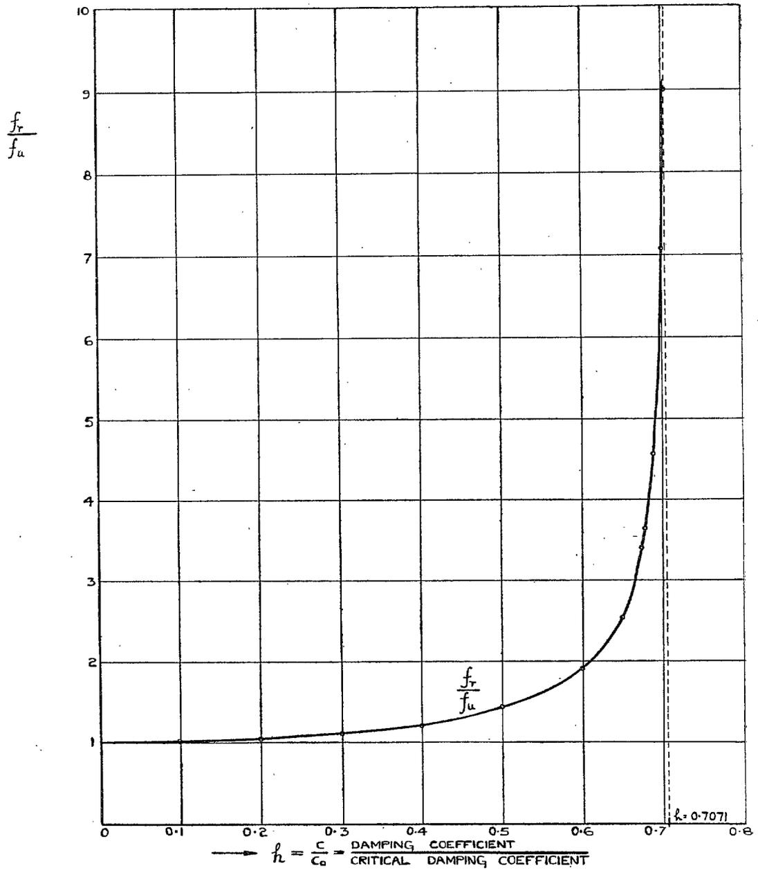
FIG. 7. - Variation of the resonant frequency of seismic type vibration pick-ups with damping.
