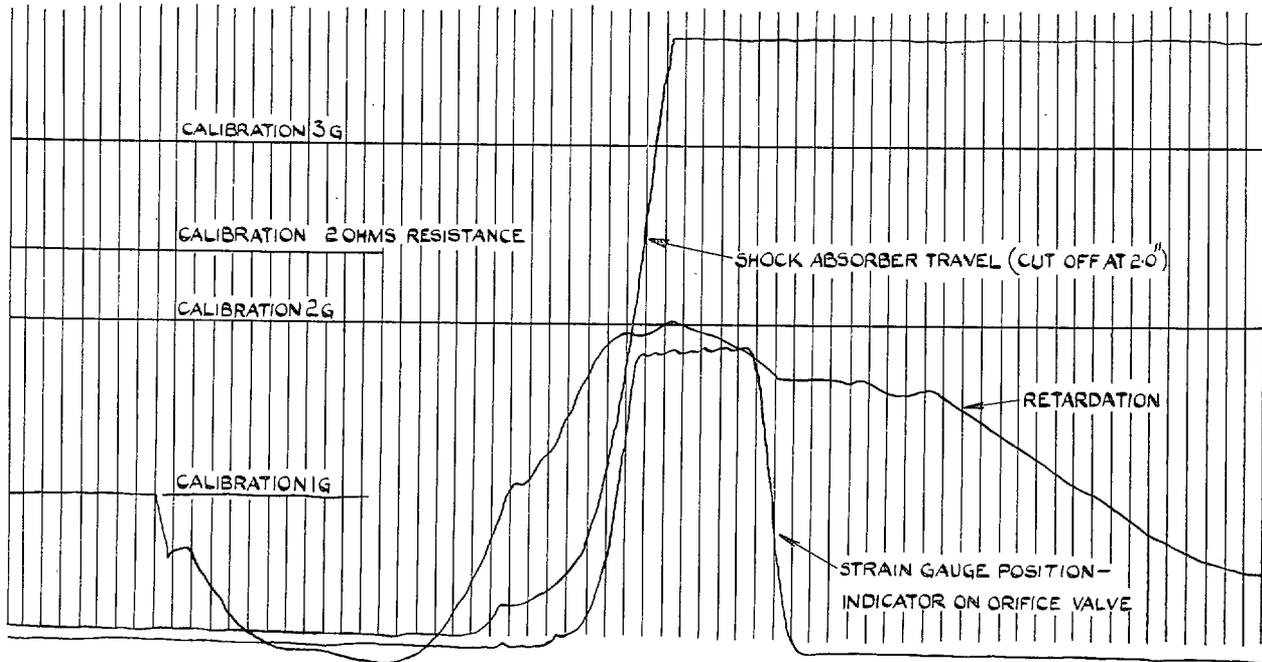
FIG. 50. Drop test on Fairey *Spearfish* undercarriage to check behaviour of orifice valve at low velocities.
