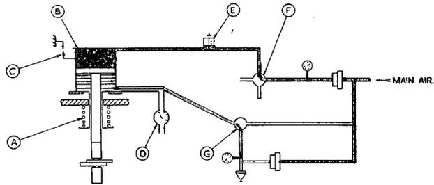
THE OPENING OF VALVE (D) EXHAUSTS AIR FROM THE UNDERSIDE OF THE PISTON THUS APPLYING A SUDDEN INCREASE IN PRESSURE TO THE SHEET BEING WELDED, I.E. A FORCE IS APPLIED. AFTER VALVE (D) HAS OPENED THE AIR PRESSURE STILL INCREASES ON THE TOP SIDE OF THE PISTON UNTIL IT REACHES A PREDETERMINED VALUE WHEN PRESSURE SWITCH (E) CLOSSES SO OPERATING VALVES (D) (F) & (C)
