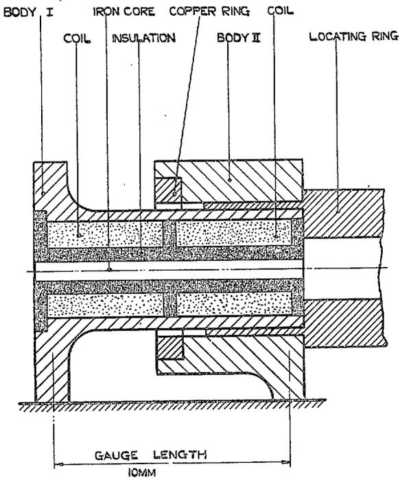
FIG. 15c. Eddy current type inductance strain unit.
