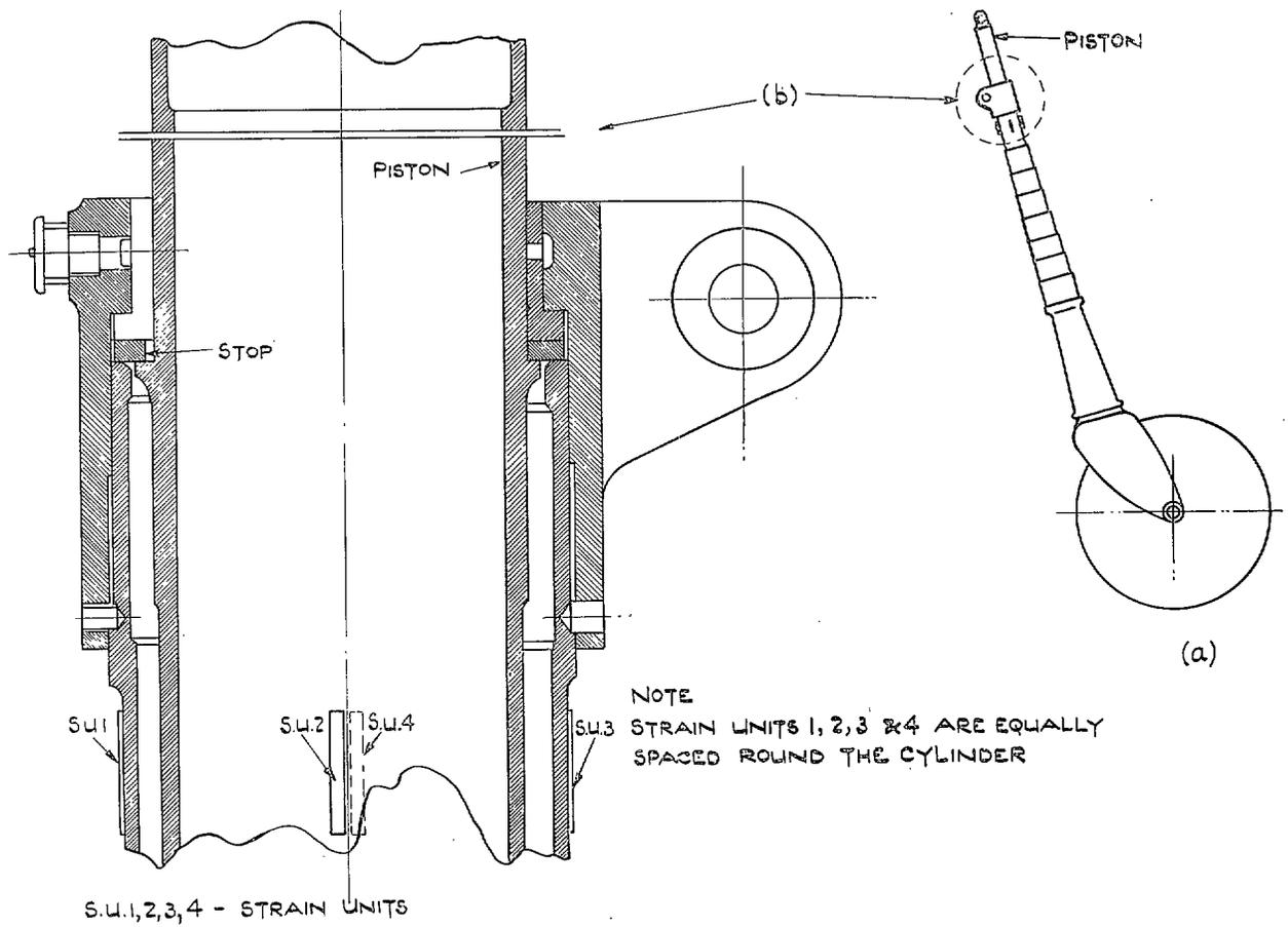
FIG. 52. Diagrams showing strain units on *Halifax* tail wheel shock absorber.
