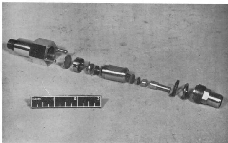
FIG. 23. Water cooled capacity type pressure pick-up unit (R.A.E.).
