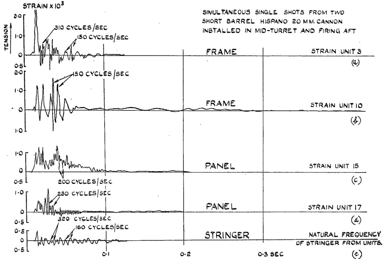
FIG. 64. Strain variations in *Lancaster* fuselage due to blast from Hispano 20 mm cannon.
