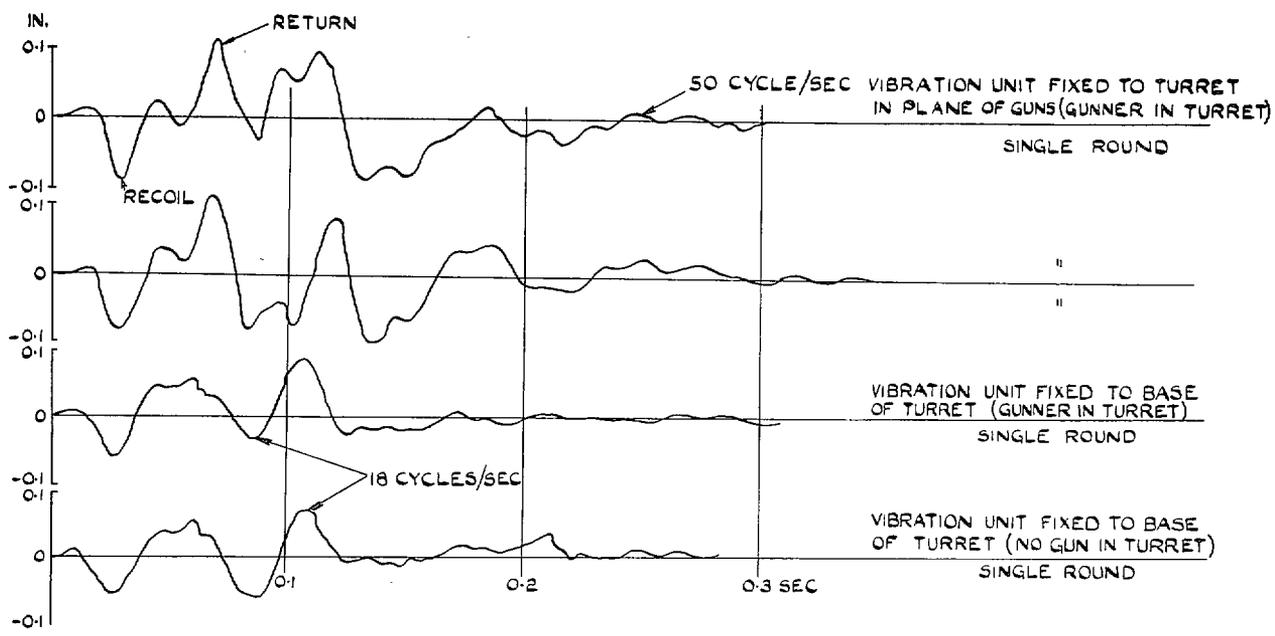
NOTE THE TWO UPPER DIAGRAMS AND THE TWO LOWER ONES ARE SHOWN TO BE IN PHASE. THIS IS PROBABLY DUE TO THE PICK-UP UNIT DIRECTION BEING REVERSED WHEN MOVED FROM TOP TO BOTTOM OF THE TURRET.
