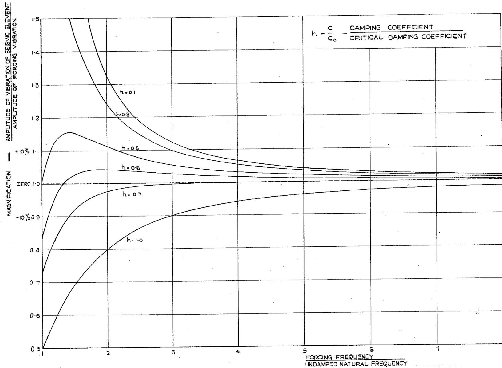
FIG. 9. Seismic pick-up variation of amplitude response with frequency for different degrees of damping.
