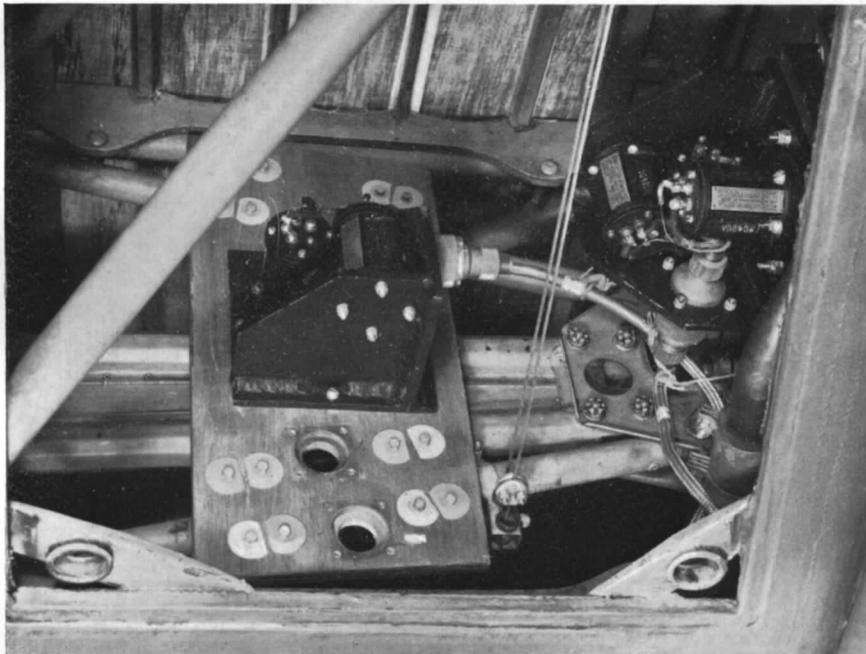
FIG. 43. Installation of vibration pick-ups in Hurricane.
