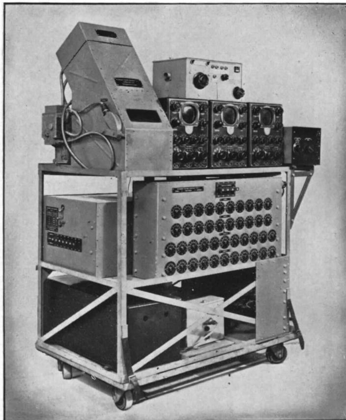
FIG. 41. Resonance testing equipment.
