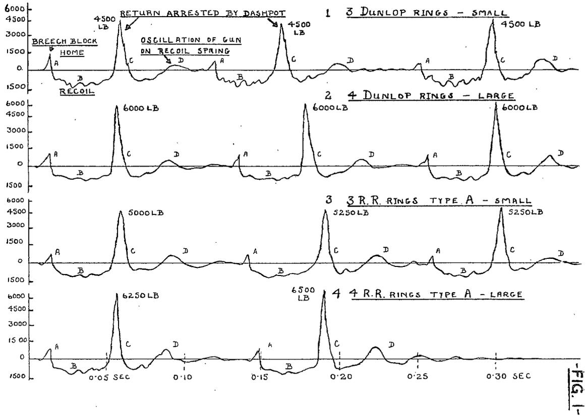
FIG. 57. Hispano 20 mm cannon. Loads on front mounting for various rubber buffers. All records taken with new rigid mounting and bevel gear feed. (Sheet I).
