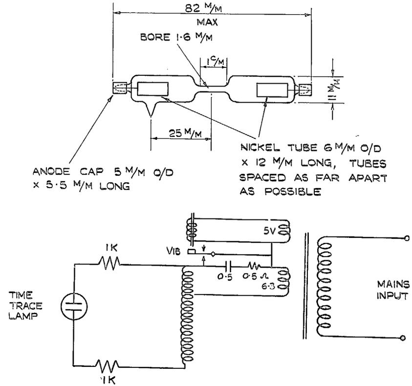
FIG. 39. Discharge lamp type T.N.1. and circuit.
