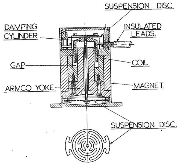
FIG. 16. Generator type pick-up unit.
