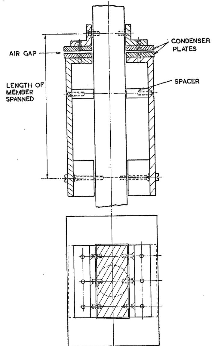
FIG. 19. Variable capacity force pick-up.
