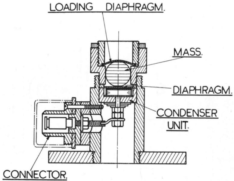
FIG. 25. Capacity acceleration pick-up, type 'B'.
