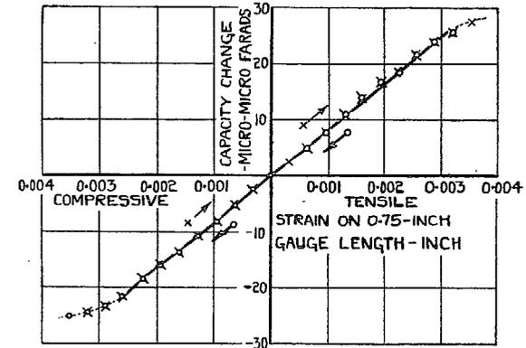
Calibration curve of multiple plate capacity strain gauge
