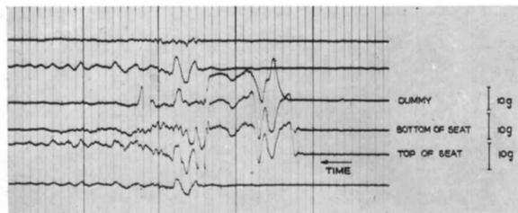
FIG. 68b. Acceleration on dummy and seat during ejection from aircraft on the ground.
