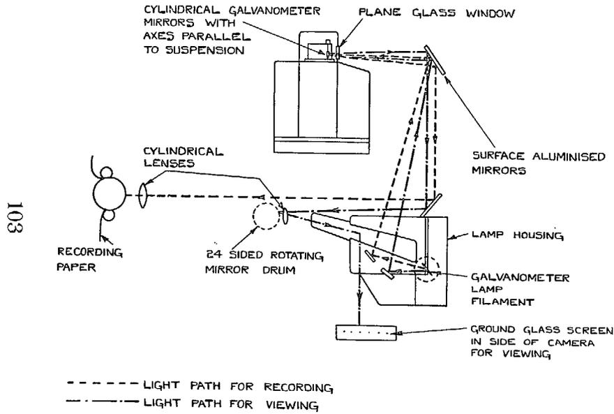
FIG. 38. Optical system of six channel vibration galvanometer camera.
