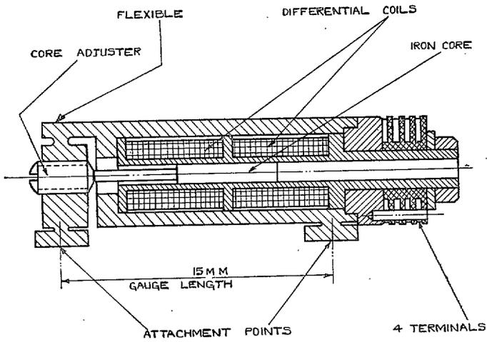
FIG. 15a. Moving core type inductance strain unit.
