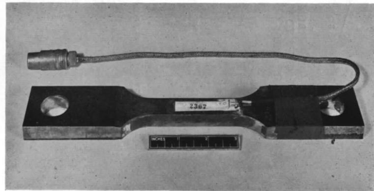
FIG. 28. Variable resistance force pick-up.
