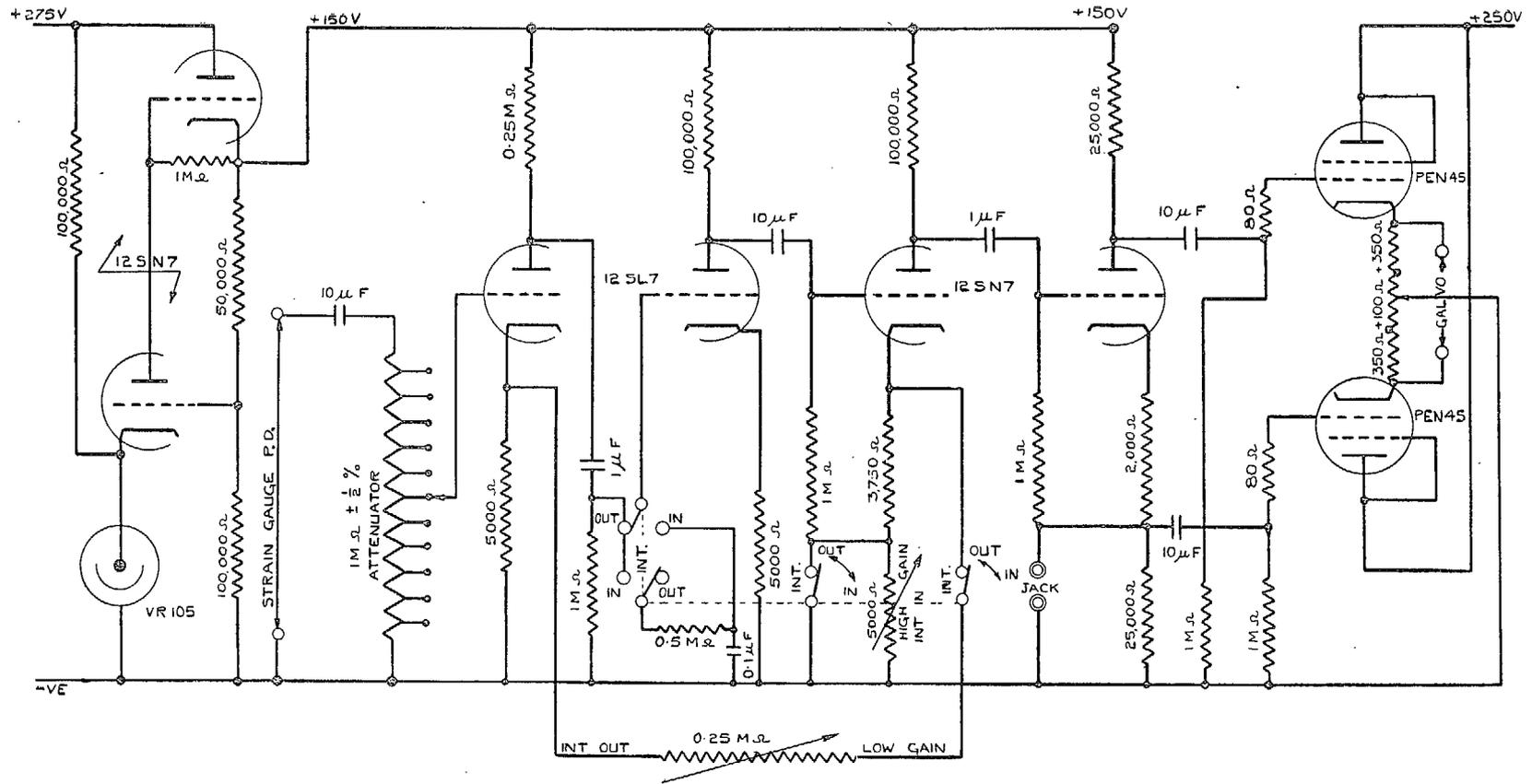
FIG. 31. Low-frequency amplifier for use with vibration galvanometer.
