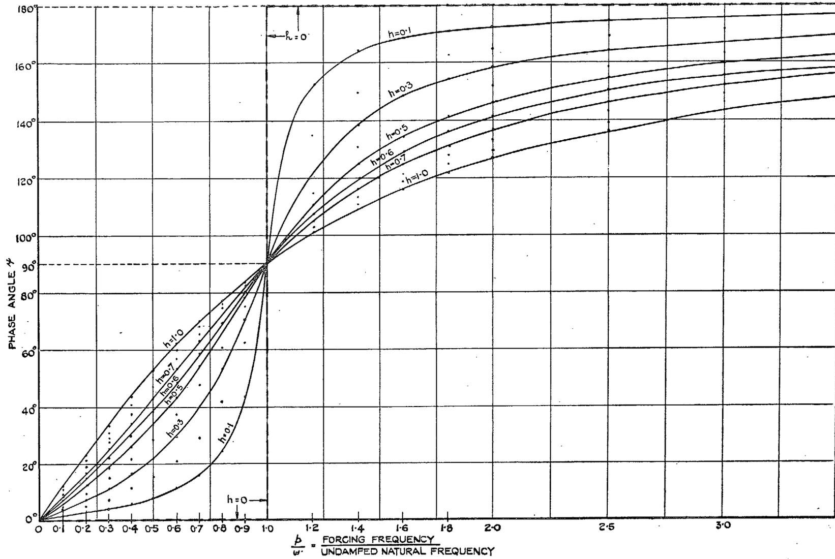
FIG. 4. Variation of phase angle with damping for a mechanical system.
