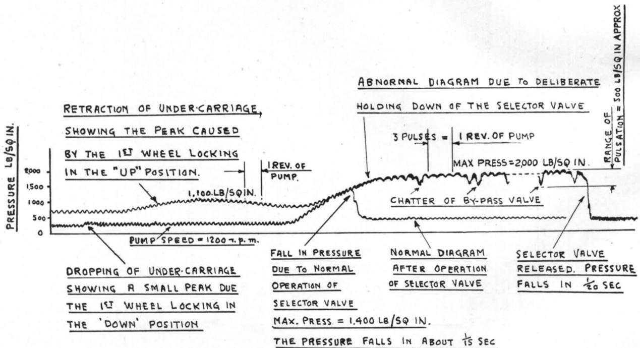
FIG. 55. Composite tracing from photographic records of pump delivery pressures taken on a Mark IV pump.
