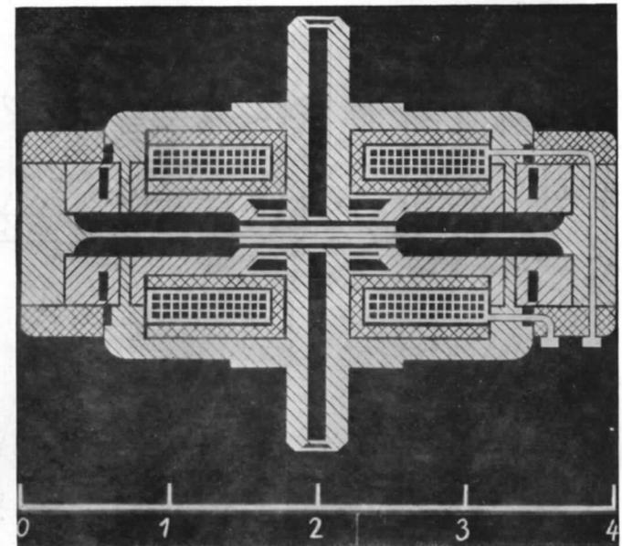
FIG. 14. Inductance type pressure unit.
