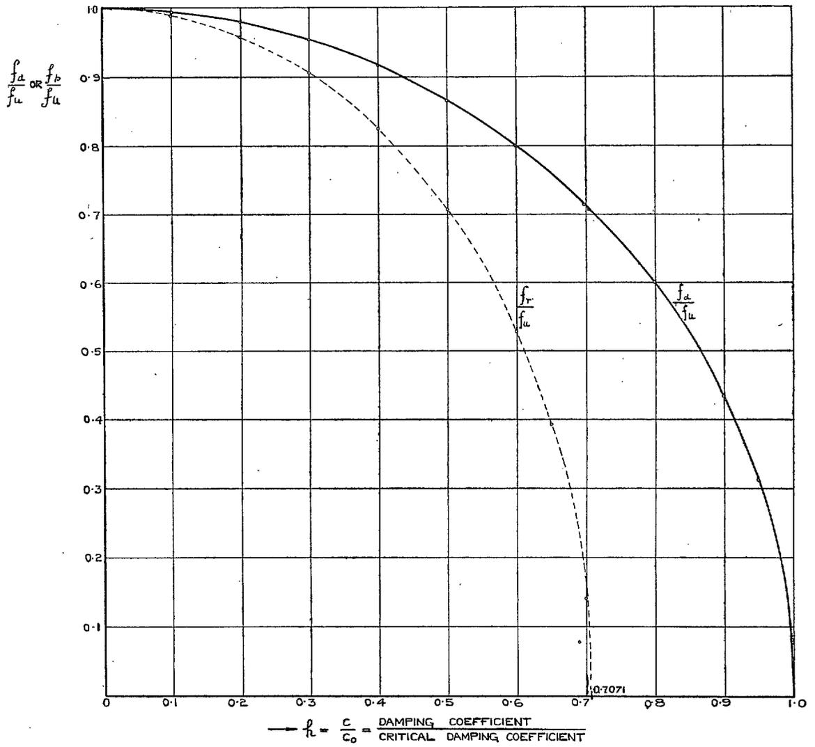
FIG. 2. Variation of damped natural frequency with damping for accelerometers, galvanometers and vibration pick-ups, and variation of resonant frequency with damping, for accelerometers and galvanometers.
