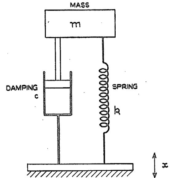
FIG. 6. Mechanical system for seismic vibration pick-up.
