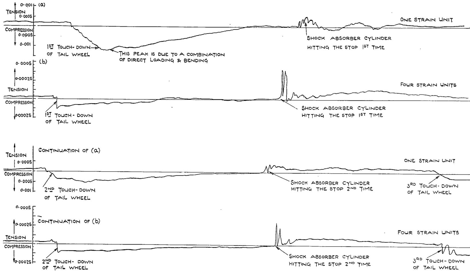
FIG. 53. Strain variations on *Halifax* tail wheel shock absorber cylinder due to butting the stop on run out.
