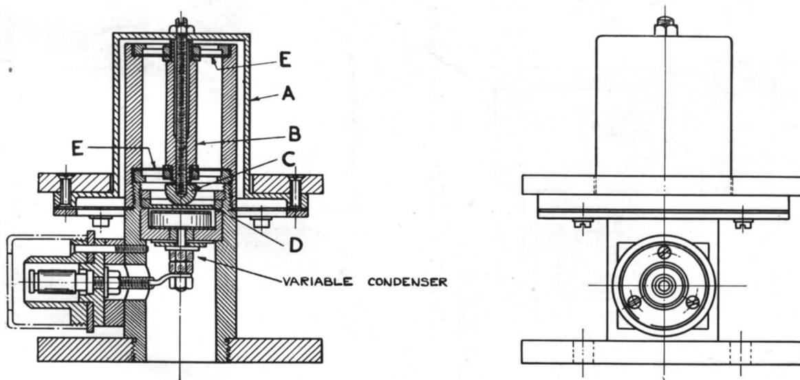
FIG. 24. Variable capacity type acceleration pick-up (low g).
