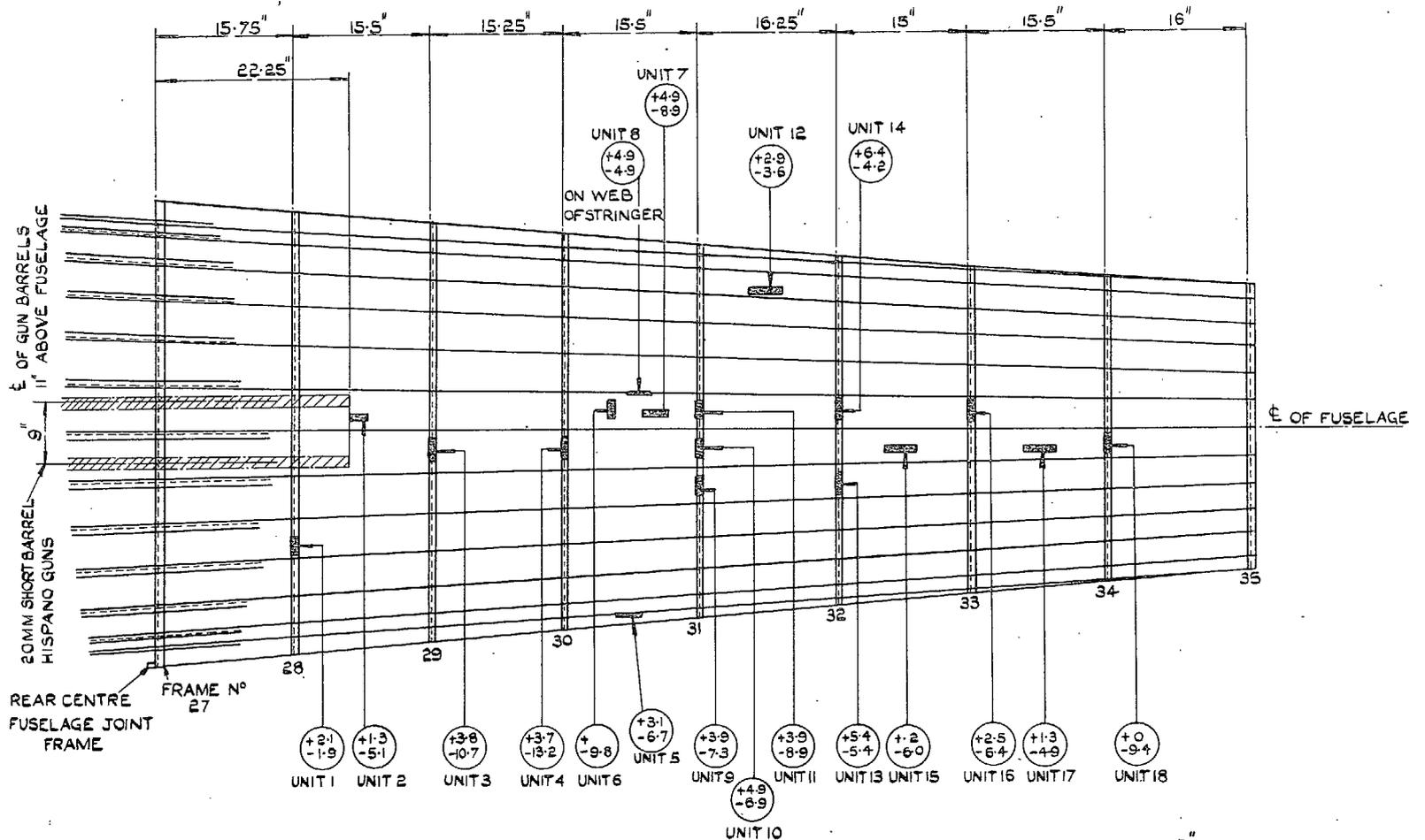
FIGURES IN CIRCLES INDICATE PEAK POSITIVE & NEGATIVE STRESS IN TONSPER SQ IN. IN A LANCASTER FUSELAGE DUE TO BLAST PRESSURE WHILE FIRING SIMULTANEOUSLY TWO 20 M M SHORT BARREL HISPANO GUNS.
