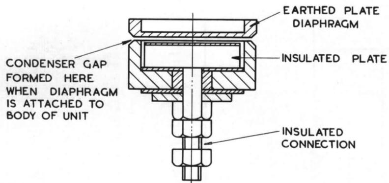
FIG. 22. Basic form of variable capacity pressure pick-up.
