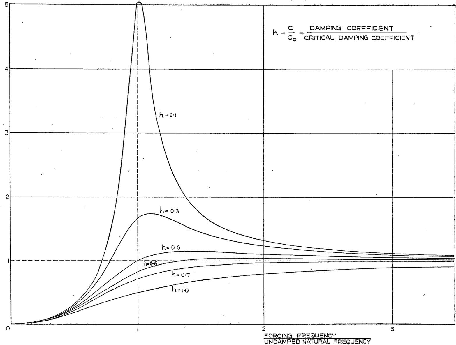
FIG. 8. Seismic pick-up variation of amplitude response with frequency for different degrees of damping.
