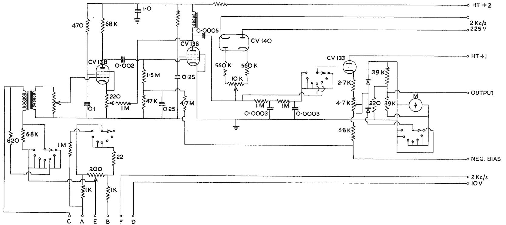
FIG. 35. Carrier amplifier and demodulator.
