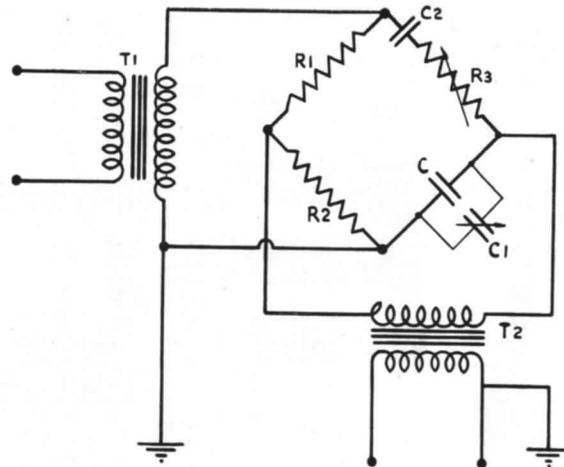
FIG. 26. Basic bridge circuit for variable capacity pick-ups.
