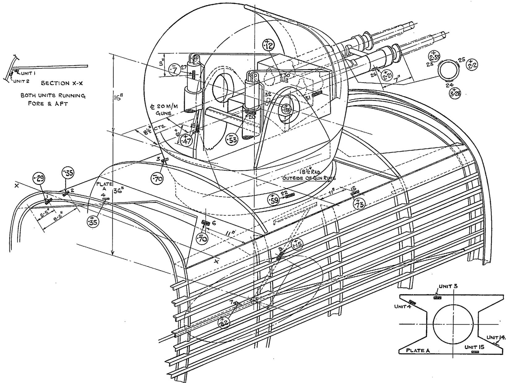
FIG. 63. Maximum stresses in *Lancaster* due to firing two 20 mm guns in the Nash and Thomson Mark II turret.
