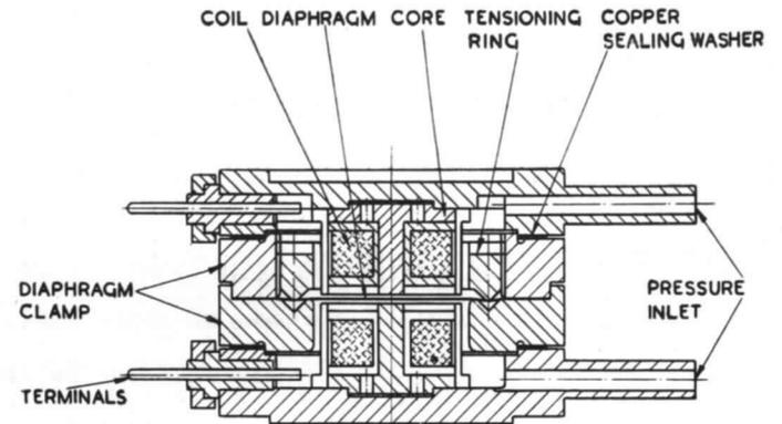
FIG. 13. Pressure pick-up—Inductance type ( $\pm 10$  p.s.i.).
