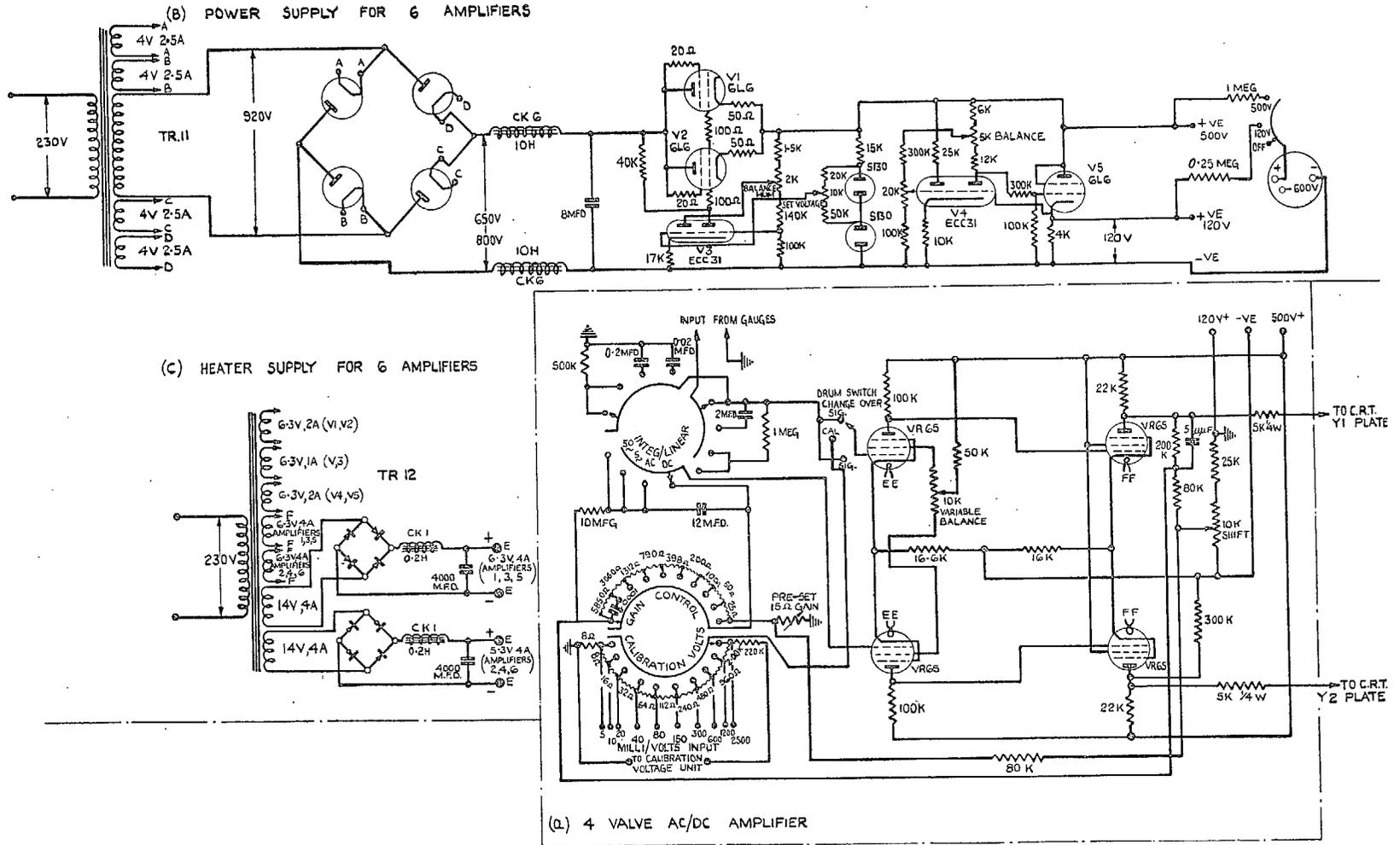
FIG. 33. Direct coupled amplifier and power pack.
