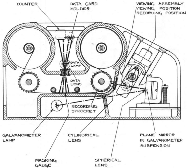
FIG. 37. Diagram of vibration galvanometer camera showing optical system.
