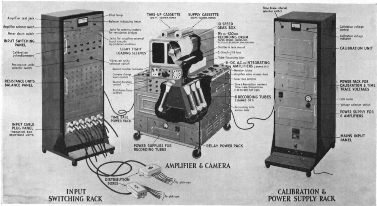
FIG. 42. Six channel cathode-ray oscillograph recording equipment (Mark I).
