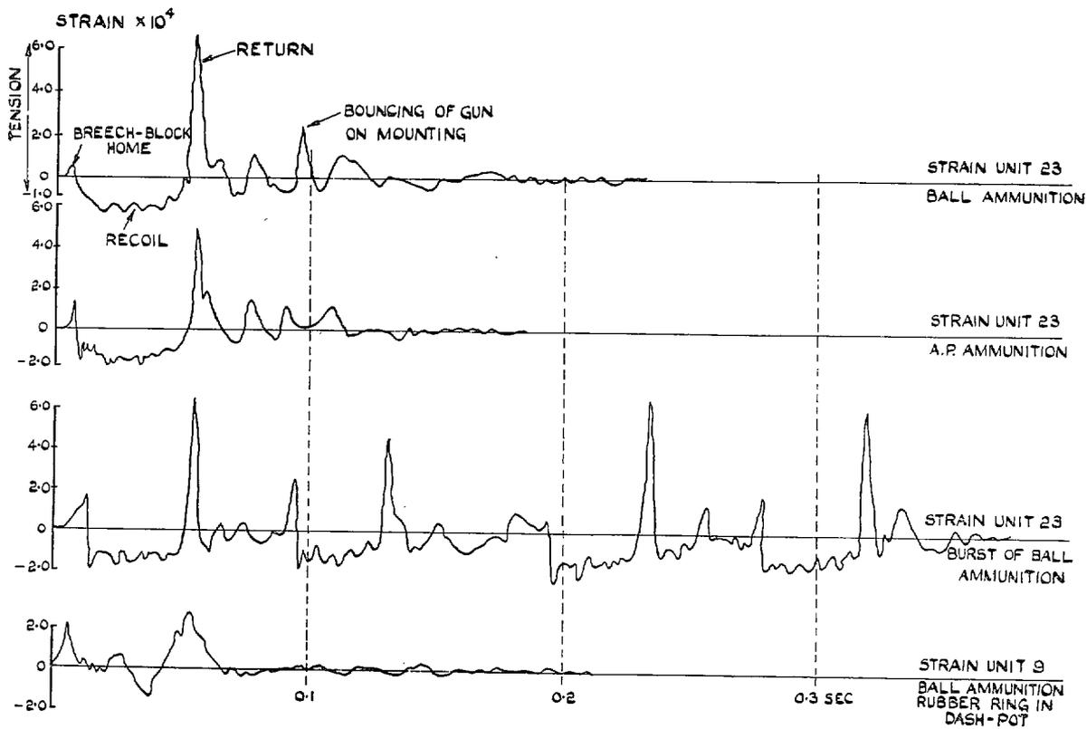
FIG. 61. Strain measurements during firing of the 20 mm Hispano cannon installed in the *Lancaster* mid-turret Mark I.
