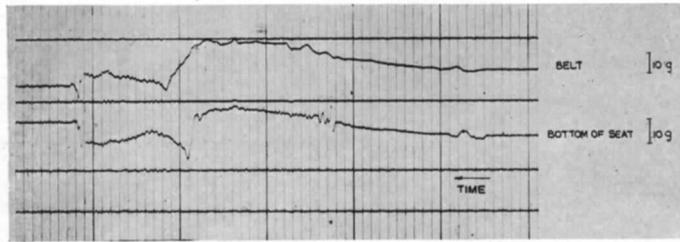
FIG. 68a. Acceleration on seat and belt on man during ejection on ground test rig.
