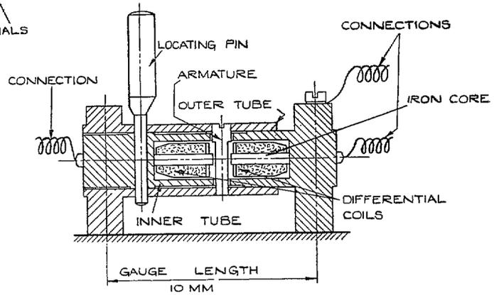
FIG. 15b. Variable air gap type inductance strain unit.
