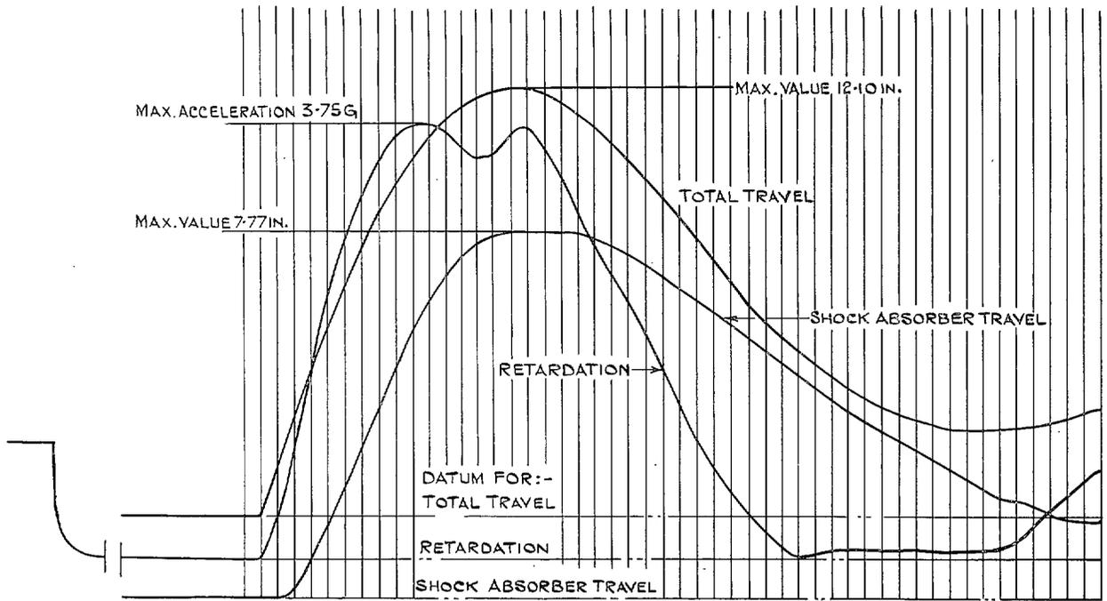
FIG. 48. Typical record taken during an undercarriage drop test.
