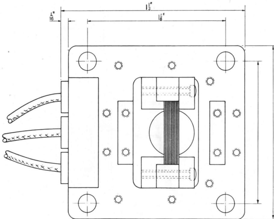
FIG. 12. Acceleration pick-up—Inductance type.
