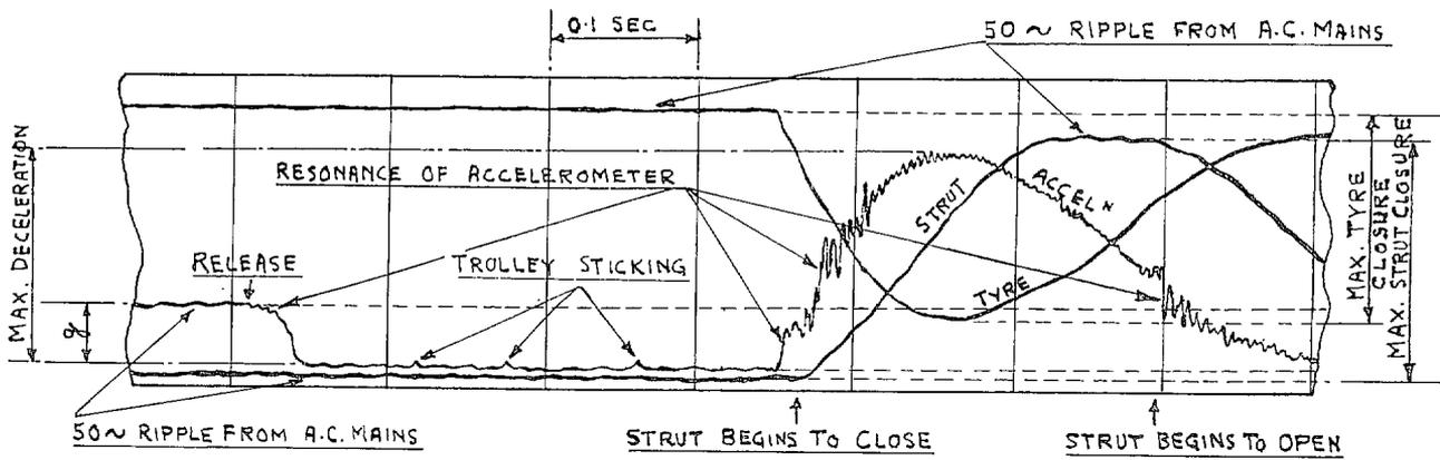
FIG. 51. Tracing of drop test records.
