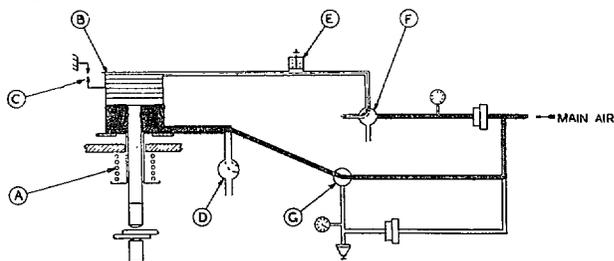
FIG. 70. Diagram showing operation of spot welding machine sequence of pneumatic cycle.
