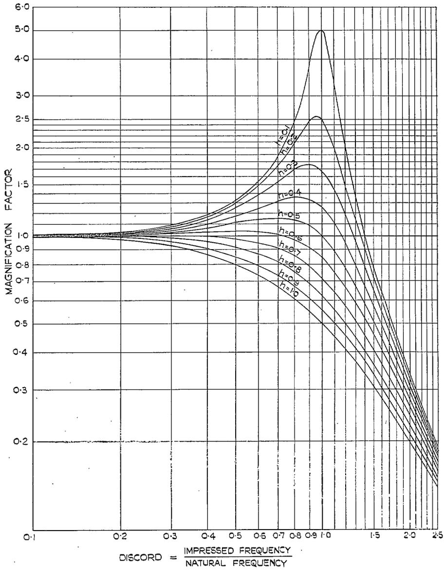
FIG. 3. Response of accelerometer system to impressed acceleration of constant amplitude.
