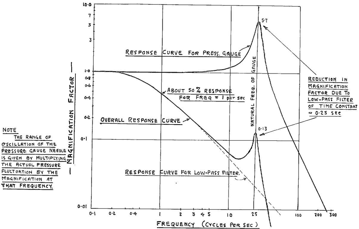
FIG. 67. Frequency response curves for oil gauge with and without low pass filter. (0 to 2,000 lb/sq in. oil gauge 2 in. diameter dial).
