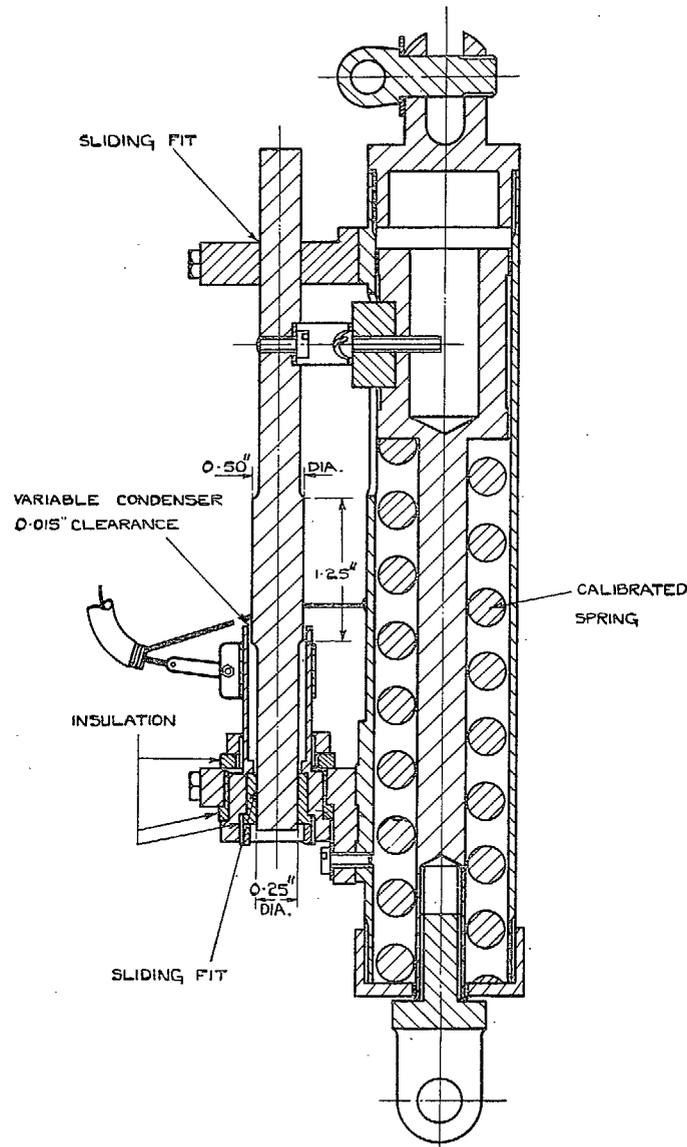
FIG. 20. Force pick-up—for glider tow rope.
