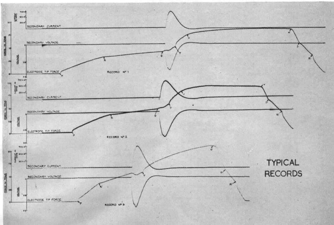
FIG. 69. Characteristics of light alloy spot welding machines. Typical records.
