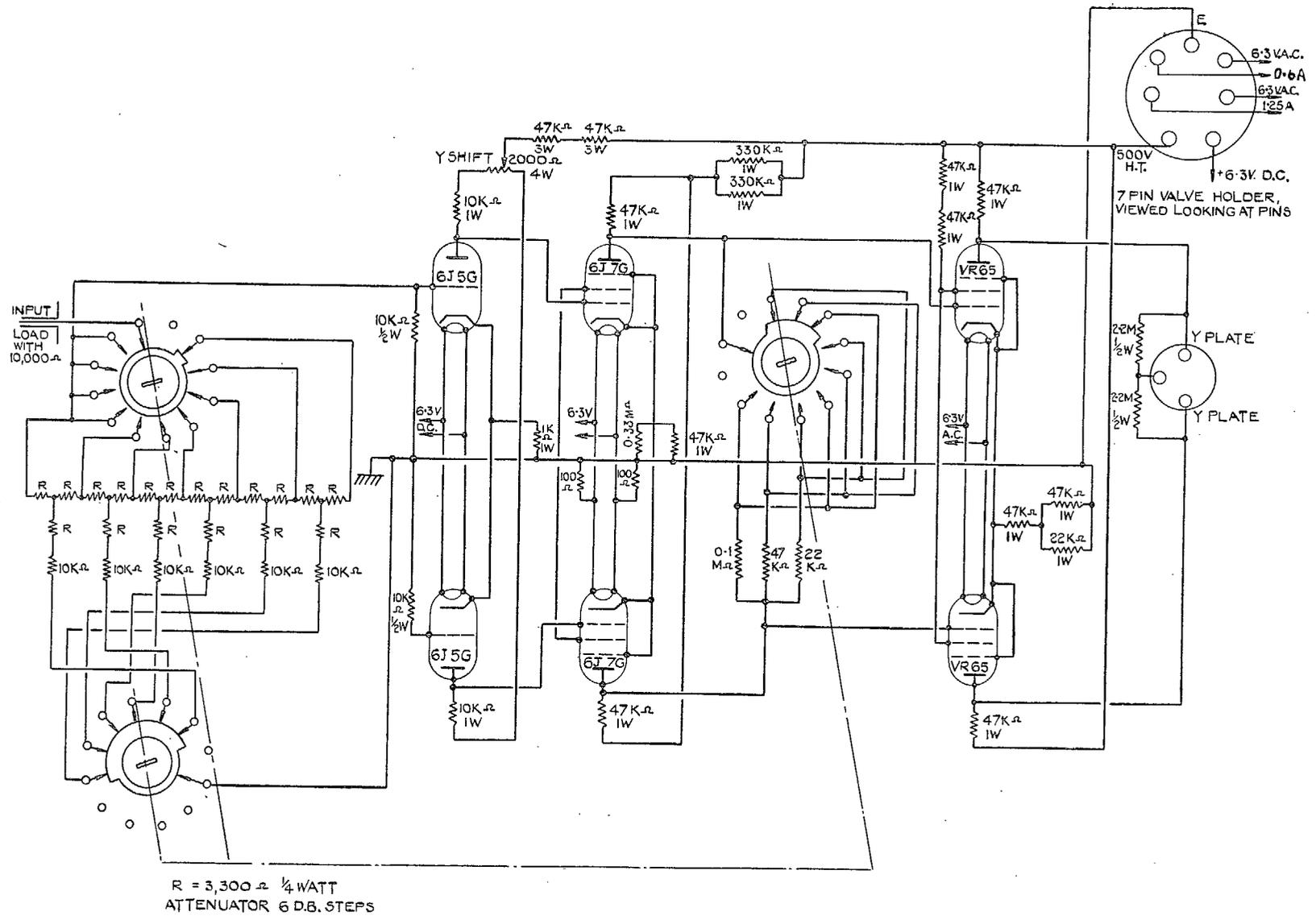
FIG. 34. Direct coupled amplifier (Plessey).
