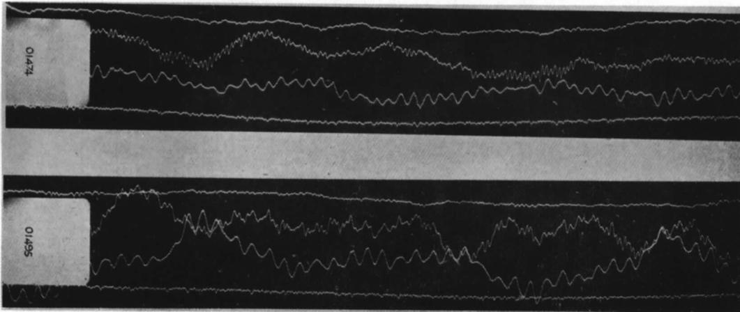
FIG. 46. Vibration characteristics of *Hurricane* in flight.
