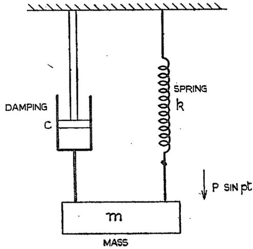
FIG. 1. Mechanical system of acceleration pick-up.
