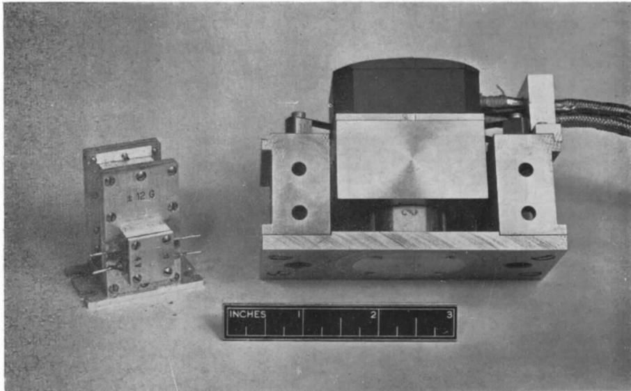
FIG. 30. Acceleration pick-ups.
