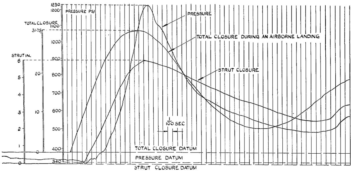
FIG. 49. Windsor T.W. unit. Variation of air pressure.
