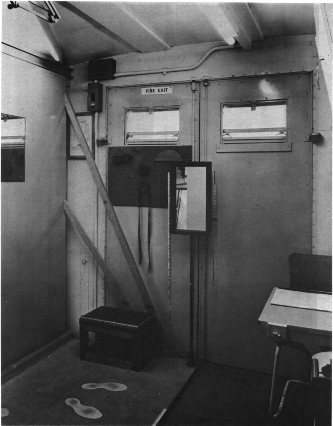
FIG. 5. Interior of laboratory showing mirror set in back wall of rig and mirror mounted on a stand for use when taking measurements in head measuring rig.
