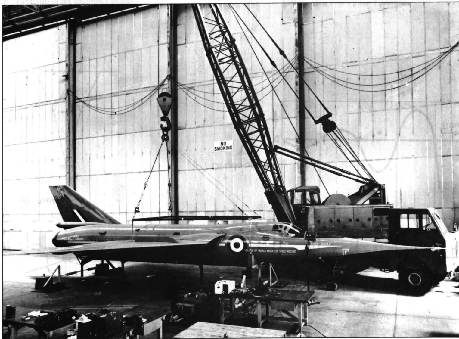
FIG. 2. Rig with spreader frame used for the Fairey Delta 2 inertia measurements.
