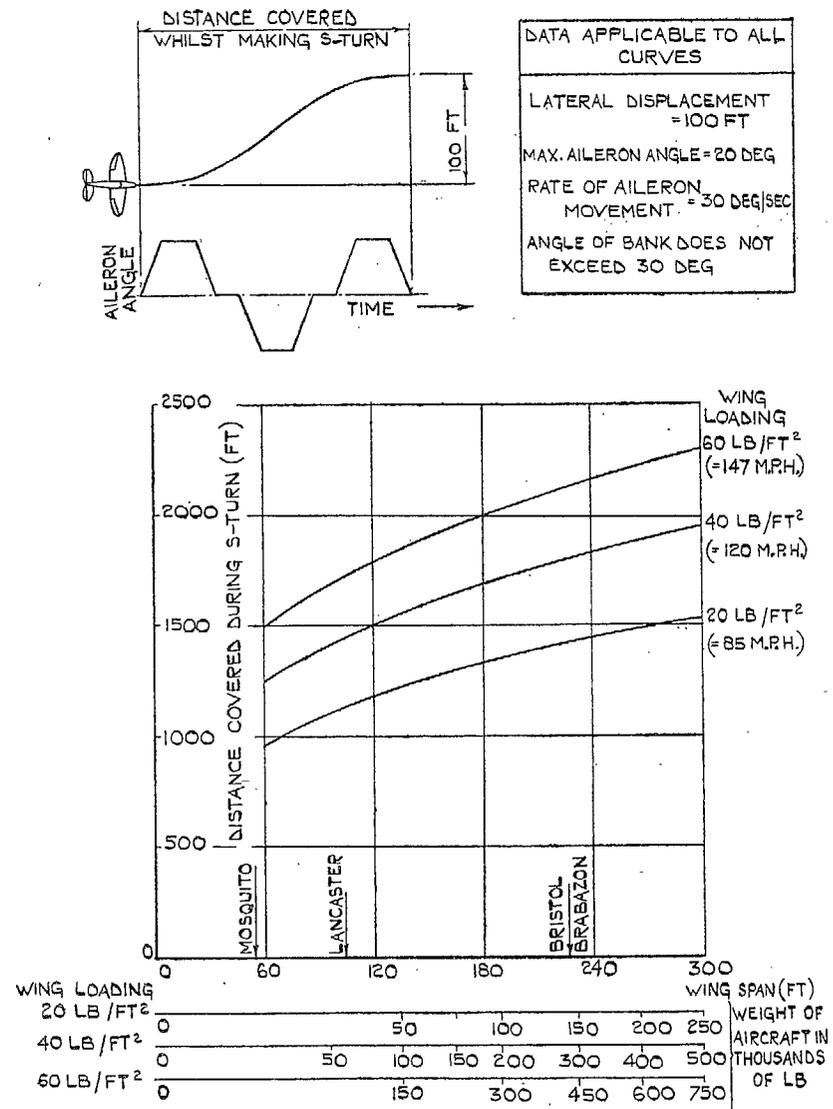
FIG. 2. Effect of aircraft size, etc. on distance travelled whilst making an S-turn.
