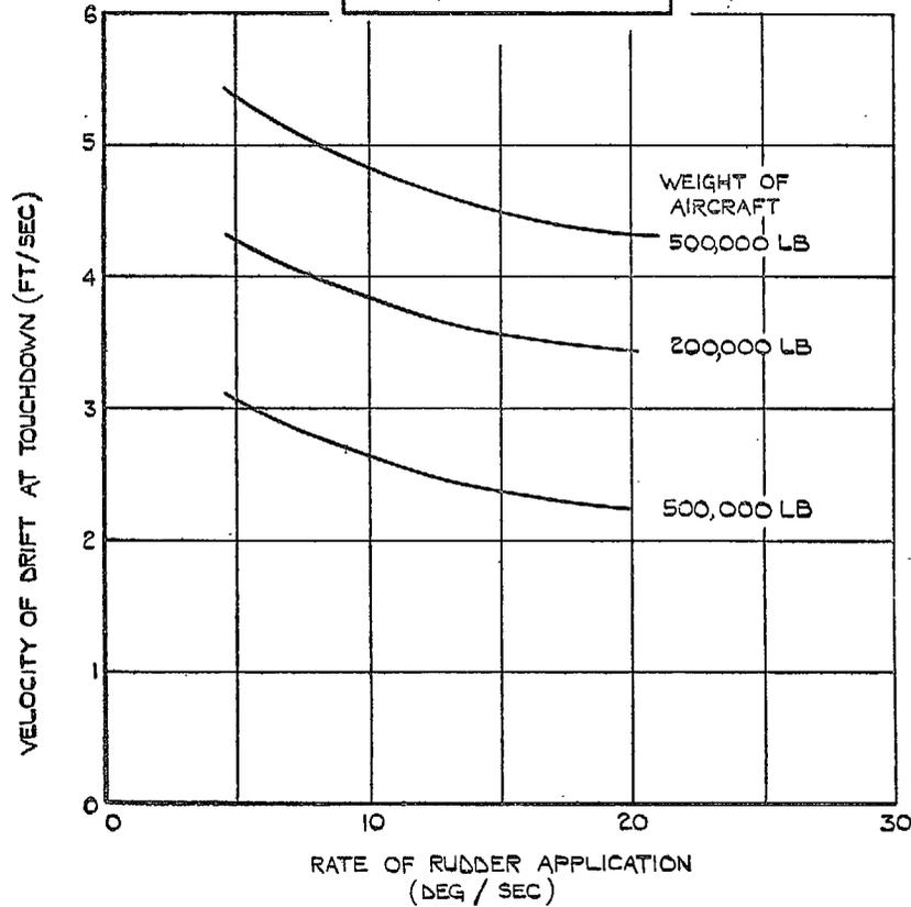
FIG. 10. Effect of rate of rudder application on lateral velocity acquired whilst making a correction for drift during approach in a 20 m.p.h. crosswind.
