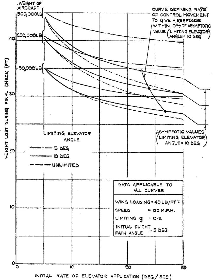
FIG. 6. Effect of initial rate of elevator application on height to start hold-off.
