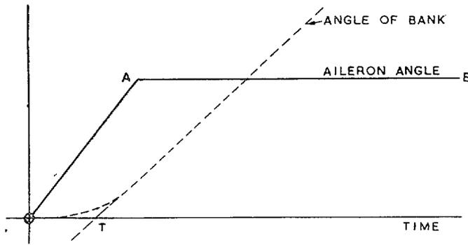
This action will produce a build-up of bank (shown dotted) which, after a short time, becomes linear.
