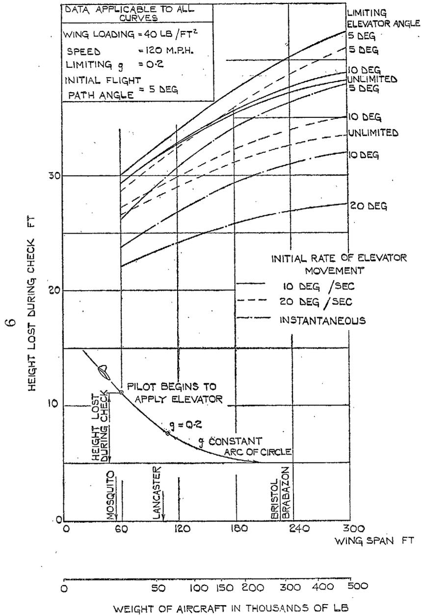
FIG. 1. Effect of aircraft size, etc. on height to start hold-off.
