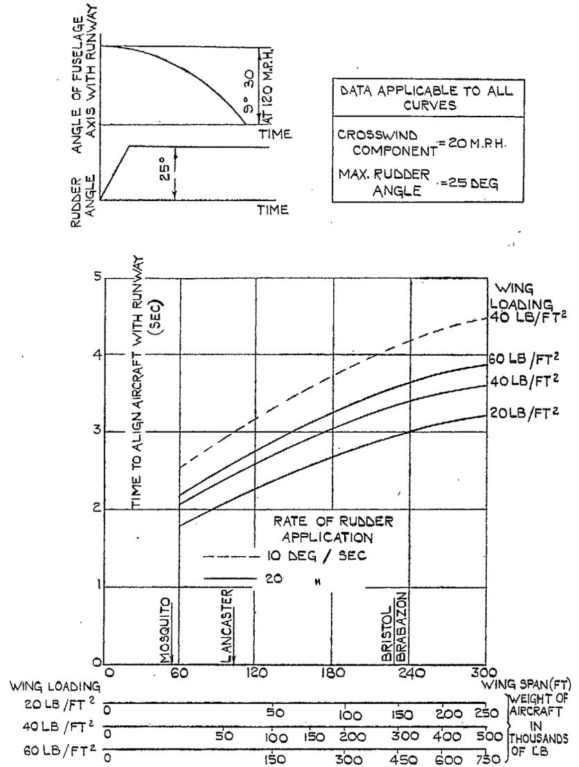
FIG. 4. Effect of aircraft size, etc. on time to correct for drift during approach in 20 m.p.h. crosswind.
