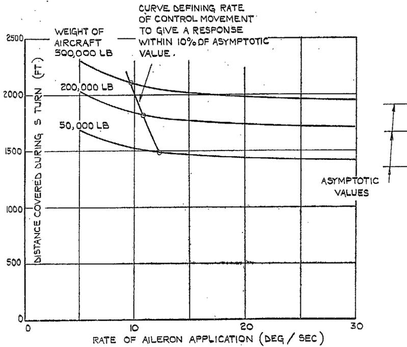
FIG. 7. Effect of rate of aileron movement on distance travelled whilst executing an S-turn.
