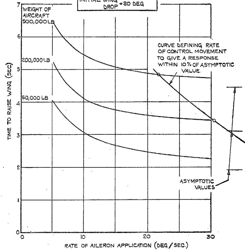
FIG. 8. Effect of rate of aileron application upon time required to correct for wing drop.
