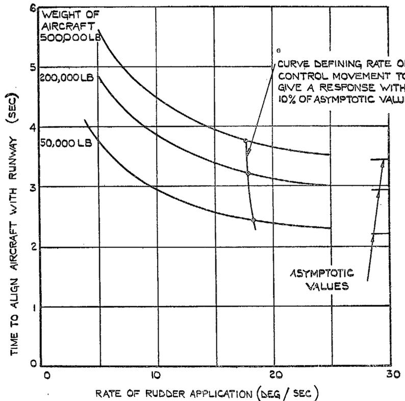
FIG. 9. Effect of rate of rudder application on time to correct for drift during approach in 20 m.p.h. crosswind.
