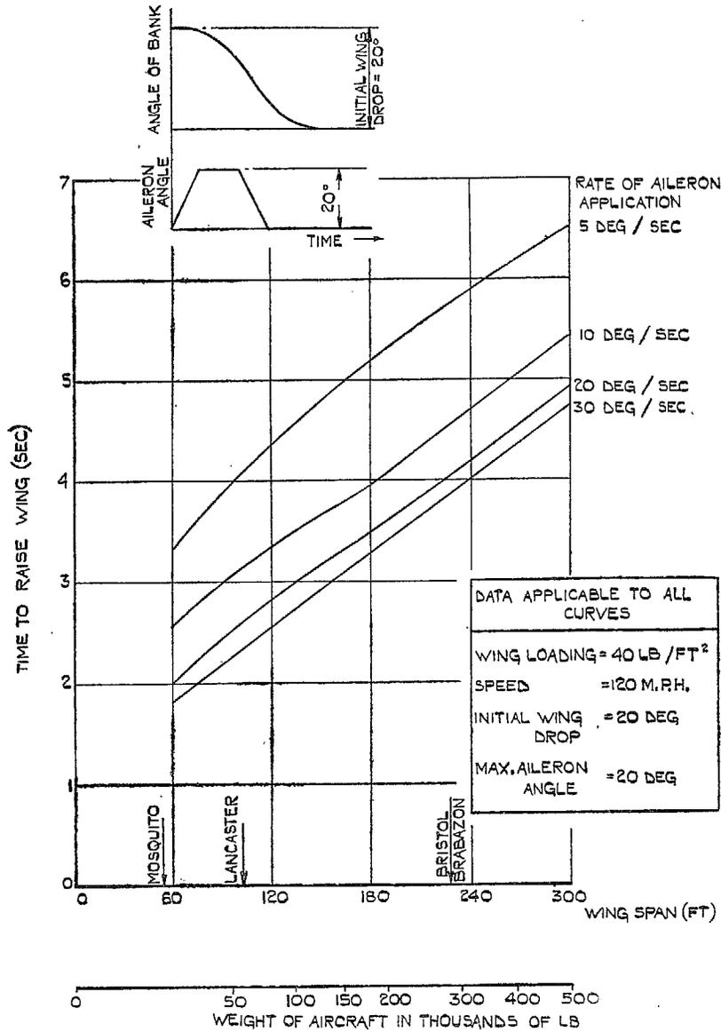
FIG. 3. Effect of aircraft size, etc. on time to correct for wing drop.
