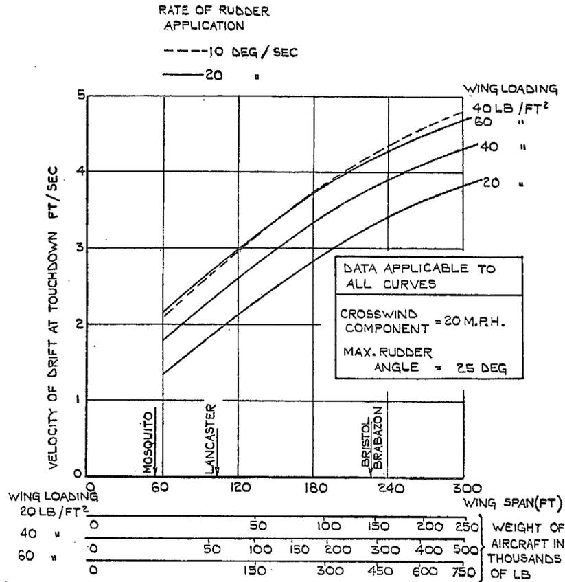
FIG. 5. Effect of aircraft size, etc. on lateral velocity acquired whilst making a correction for drift during approach in a 20 m.p.h. crosswind.
