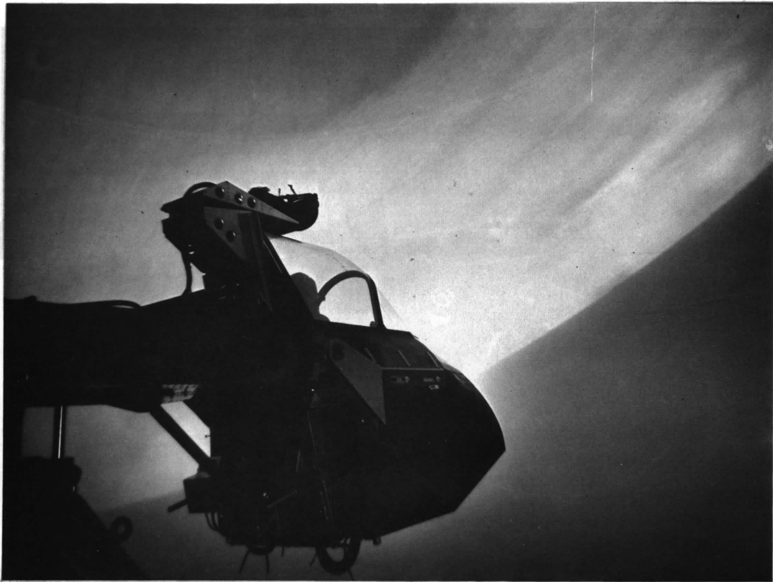
FIG. 15. Visual scene of horizon and clouds produced by the 'Skyscape' projector.
