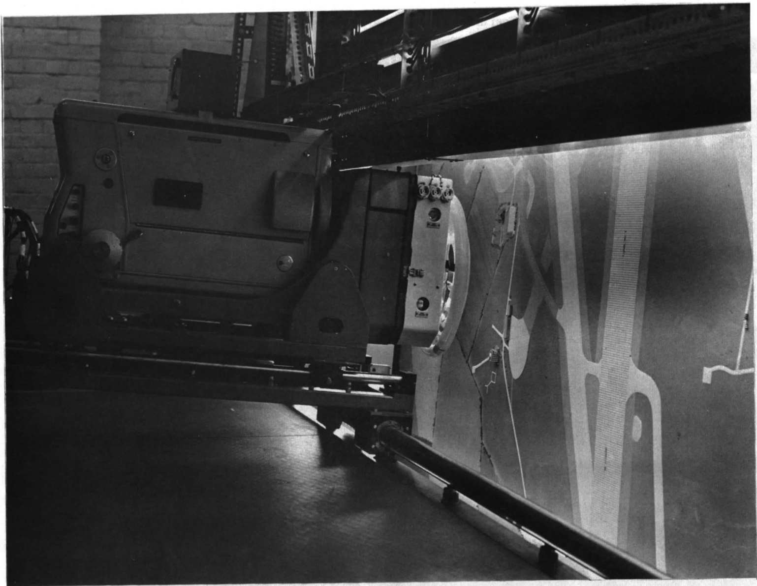
FIG. 22. Camera and airfield model used for closed circuit T.V. visual simulation system.
