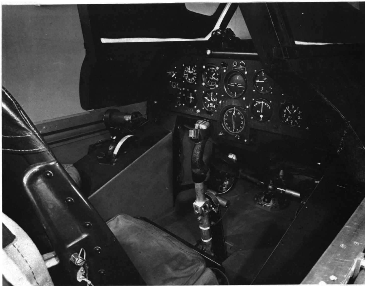
FIG. 10. Centre stick control layout in the single seat cockpit.
