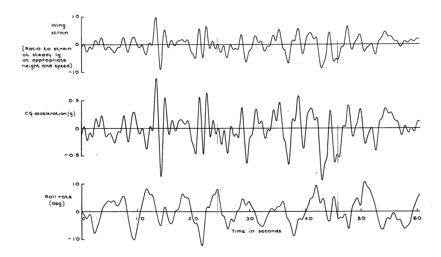
Fig. 1 Roll rate, CG acceleration, wing strain gauge output after filtering to remove frequencies above 1Hz
