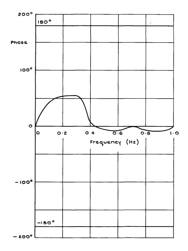
Fig. 17 Phase. Aileron angle and roll acceleration
