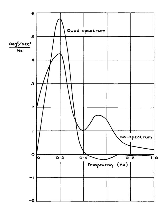
Fig. 15 Co-spectrum and Quad spectrum. Aileron angle and roll acceleration
