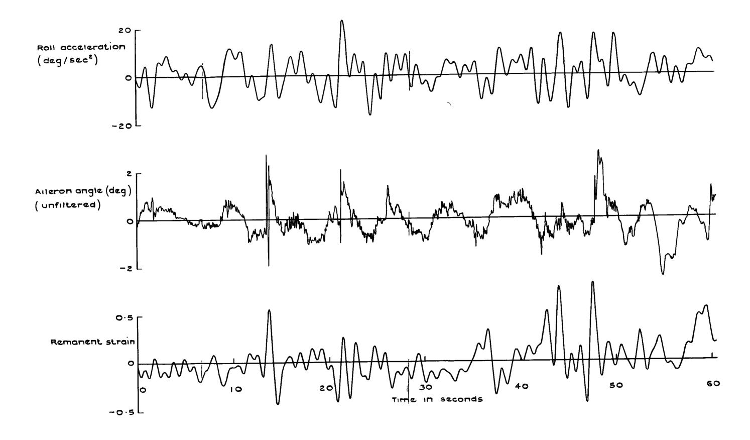
Fig.2 Remanent strain, aileron angle (unfiltered) and roll acceleration
