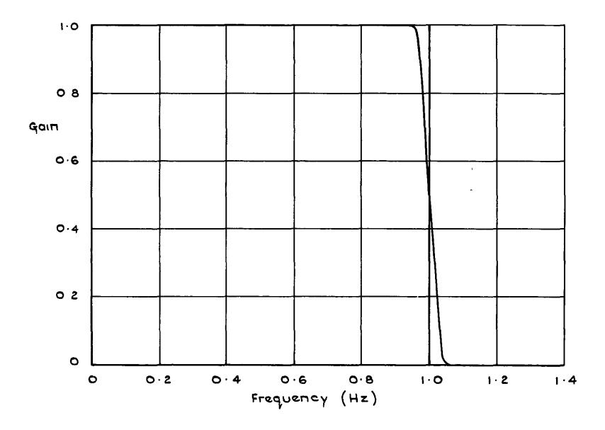
Fig.9 Filter gain. Low pass filter
