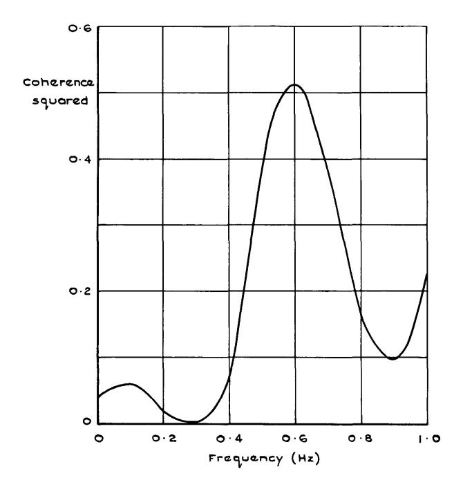
Fig.6 Coherence squared. Remanent strain and roll acceleration
