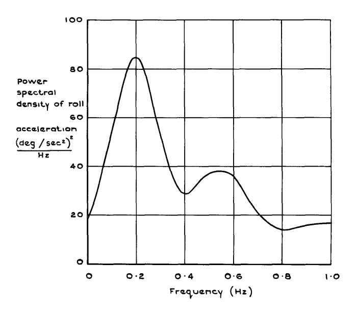
Fig.4 Power spectrum—roll acceleration
