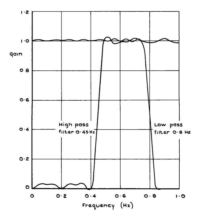
Fig. 10 High and low pass filters
