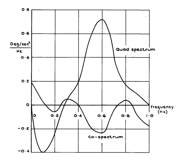
Fig. 5 Co-spectrum and Quad spectrum. Remanent strain and roll acceleration
