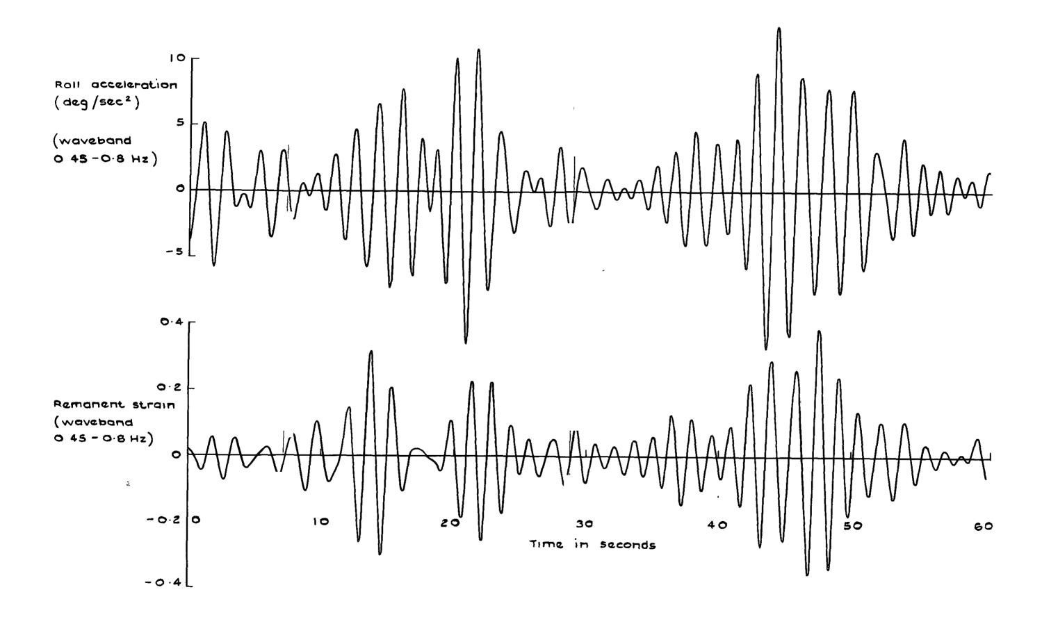
Fig. 8 Remanent strain and roll acceleration after filtering. Waveband 0.45 - 0.8 Hz
