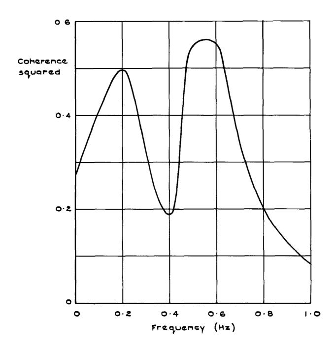
Fig.16 Coherence squared. Aileron angle and roll acceleration
