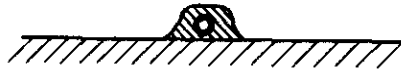
a Cross section of araldite fairing for surface tubes (Scale - full size)
